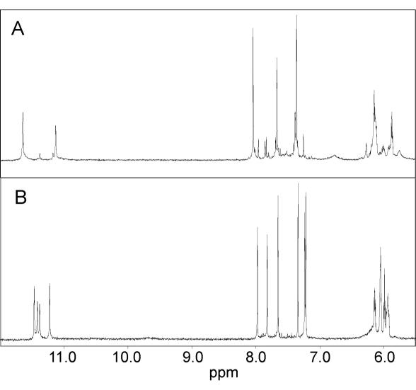
Selected regions of 1D  $^{1}$ H-NMR spectra (700 MHz) of Q33 (**A**) and Q55 (**B**) 2 mM in 0.6 ml (H $_{2}$ O/D $_{2}$ O 9:1) buffer solution having 10 mM KH $_{2}$ PO $_{4}$ , 70 mM KCl, 0.2 mM EDTA, pH 7.0 at 25°C. The guanine imino protons involved in G-tetrad formation resonate between 11.0 and 12.0 ppm. The narrow non-exchangeable base protons resonate between 7.0 and 8.0 ppm.
