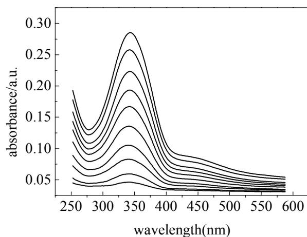
*Figure 1.* UV-Vis absorption spectra of electrostatic self-assembly azobenzene films on a quartz wafer (from bottom to top: 1 to 10 bilayers).
