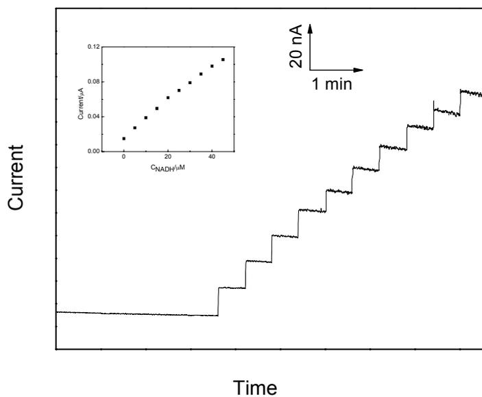
Fig. S3 Chronoamperometric curve of the steady state response at PFIL-Nafion modified glass carbon electrode in phosphate buffer solution (0.05 M, pH = 7.4) on increasing the concentration of NADH in 5 μM steps. Working potential: +0.75 V. Insert: the calibration curve for NADH at PFIL-Nafion modified GCE.
