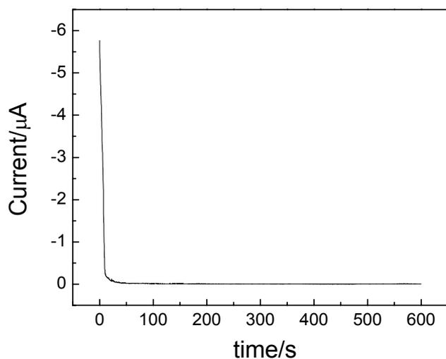
Fig. S5 Chronoamperometric response of PEI/PSS/PFIL multilayer on ITO in 10 mM NaPF<sub>6</sub> or NaCl. The potential was held at 0.3V for 600 s.
