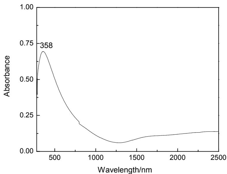
Fig. S2 UV-vis-NIR of PFIL electrodeposited onto ITO. The film of PFIL on ITO was obtained by electrophoresis at -2 V for 600 s. A strong adsorption band at 358 nm was attributed to the adsorption of imidazolium rings.<sup>[4]</sup> The result further verified the successful synthesis of PFIL, which was in agreement with FTIR data.
