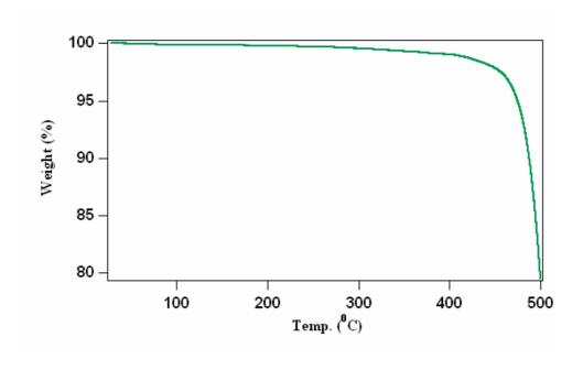
Fig. SI (1): TG analysis for 1 over the temperature range from 25- 500°C at a heating rate of  $\beta = 5$ °C /min under the N<sub>2</sub> atmosphere.
