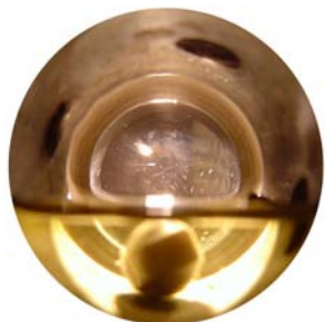
Fig. 3a Phase behavior during carbamate formation (130 °C, 120 – 130 bar): biphasic mixture with supercritical-like CO 2 phase (top) and CO 2 -rich liquid phase (bottom).
