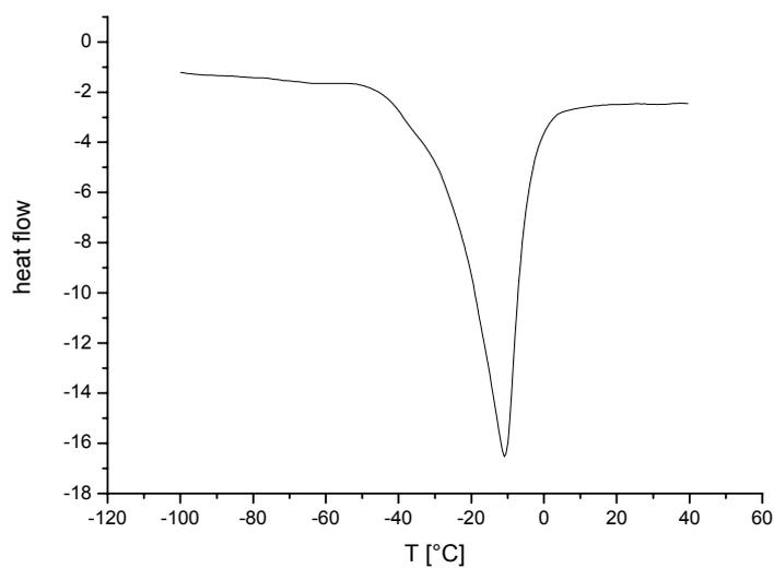
**Figure S8: DSC of Ethyldimethylsulfonium dicyanamide**
