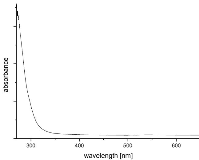
**Figure S6: UV/Vis-absorbance of neat Trimethylsulfonium dicyanamide**
