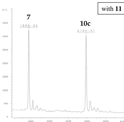
**Figure S7.** MALDI TOF spectrum from primer extension with template **8g**, primer **7** and downstream-binding trimer **11**, using **6c** (20 mM) at pH 8.9, after 20 h at 4 °C. Peaks at slightly higher mass than those of the pseudomolecular ion labeled are caused by salt adducts ( $\text{Na}^+$ ,  $\text{K}^+$ ,  $\text{Mg}^{2+}$ ).
