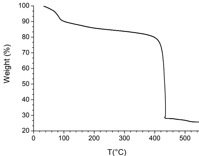
**Figure S1a:** TGA of MIL-88B under O<sub>2</sub> atmosphere.
