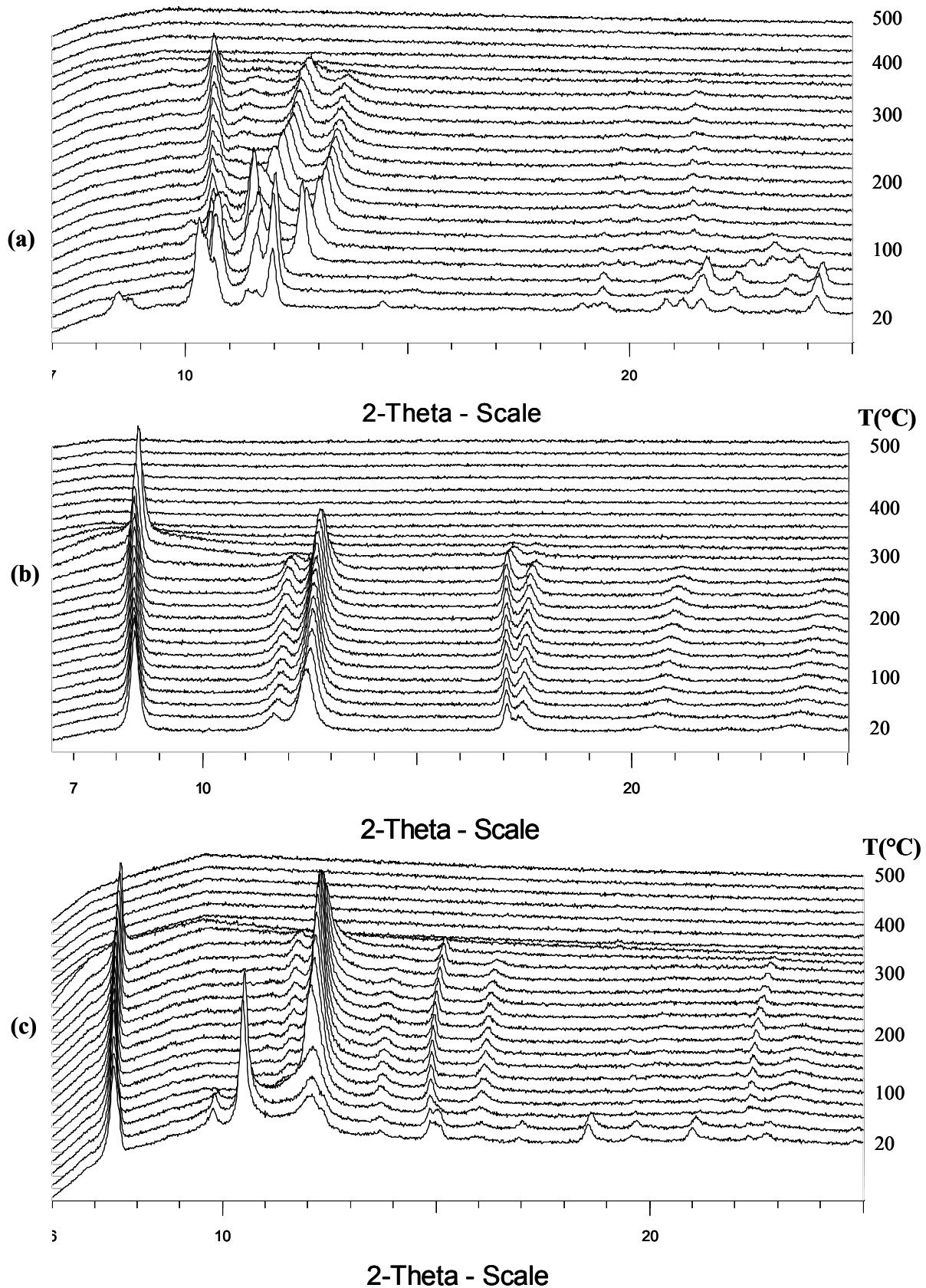
**Figure S2:** X-Ray thermodiffractometry of MIL-88B, C, D under air atmosphere.
