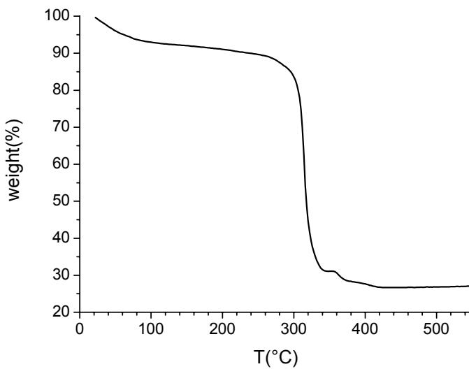
**Figure S1b:** TGA of MIL-88C under O<sub>2</sub> atmosphere.
