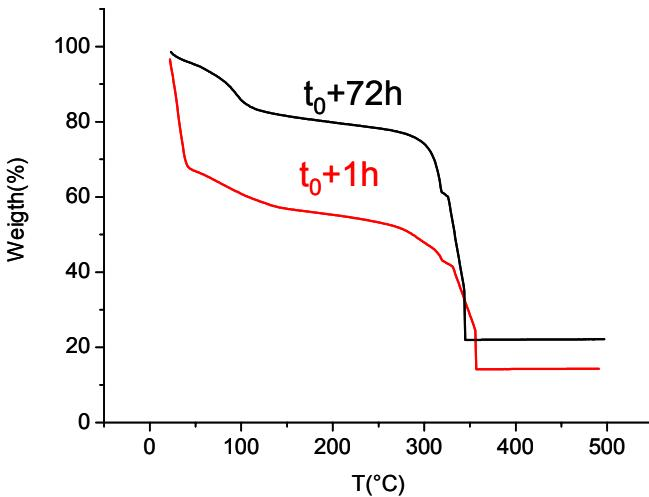
**Figure S1c:** TGA of MIL-88D performed under O<sub>2</sub> atmosphere dried a few hours at room temperature. Bottom (red): after one hour; Top (black): after 3 days.  $T(^{\circ}\text{C})$
