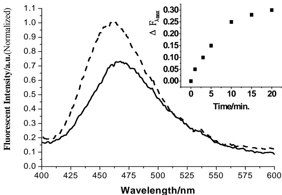
**Figure S6b** Fluorescent spectra (excited at 355 nm) of the BTE-NA-(chol)<sub>2</sub> gel, the open-ring isomer (—), in the photostationary state(-----) (0.5 wt/v %) upon irradiation by 365nm light at room temperature. Inset curves show the fluorescent change value at maximum emission wavelength with irradiation times.
