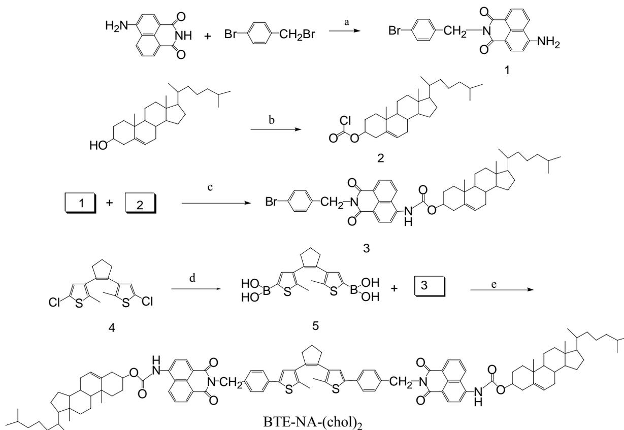
**Scheme S1** The synthetic routes of BTE-NA-(chol)<sub>2</sub> gel. (a) NaOCH<sub>3</sub>, DMF, at room temperature, 24h, 85% yield; (b)(COCl<sub>2</sub>)<sub>3</sub>, CH<sub>2</sub>Cl<sub>2</sub>, 0-20°C; (c) Dioxane, Et<sub>3</sub>N, reflux, 24h, 53% yield; (d)n-BuLi, -78°C, B(OBu)<sub>3</sub>, HCl, 63.8% yield; (e) Pd(PPh<sub>3</sub>)<sub>4</sub>, 20%NaCO<sub>3</sub>, THF, 60°C, 21% yield.
