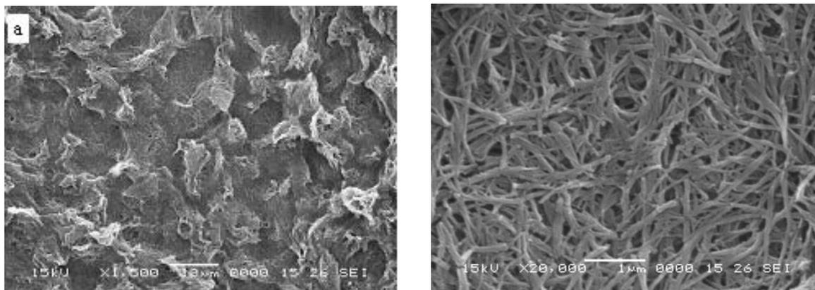
**Figure S3.** SEM images of BTE-NA-(chol)<sub>2</sub> gel (The gels were prepared from the toluene/Ethanol(1:3v/v), [BTE-NA-(chol)<sub>2</sub>]=0.5 wt %).
