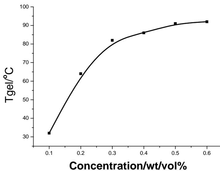
**Figure S4** Gel-to-sol phase transition temperature as the BTE-NA-(chol)<sub>2</sub> concentration in mixed solvent of the toluene/1-butanol (1:3v/v).
