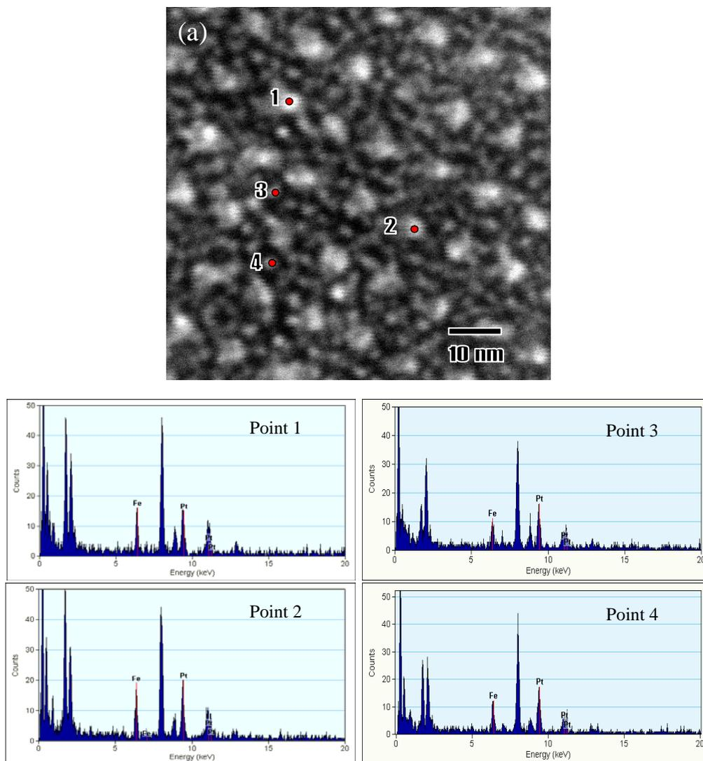
STEM micrograph and EDX spectra of AB<sub>13</sub> nanoparticle superlattice. Panel (a) shows the image recorded under STEM mode. The EDX spectra recorded from positions 1, 2, 3, and 4 are shown in (b) – (e) respectively. Under STEM mode, the spot size can be controlled to less than 0.5 nm, which guarantees that the measured spectra only come from each single particle.
