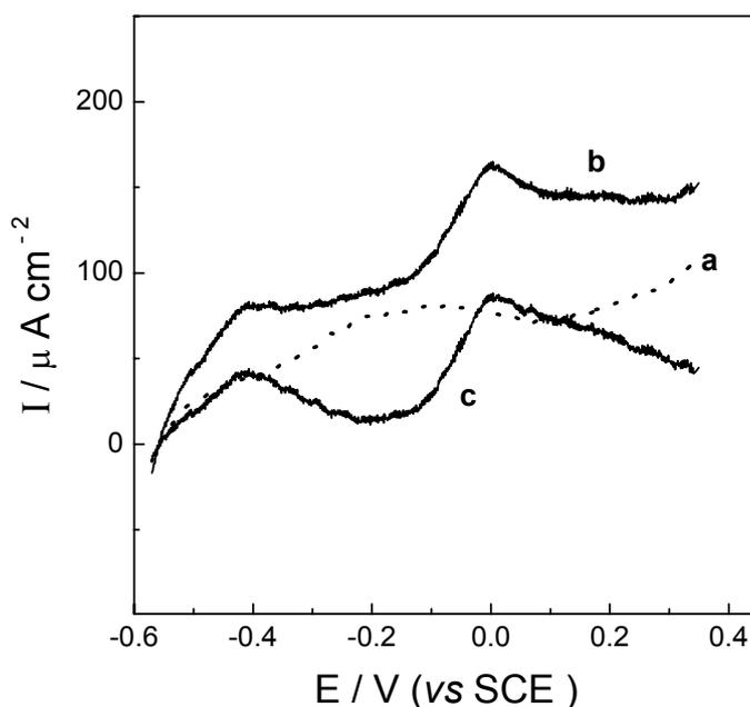
The current-potential curves obtained on a graphite-PTFE composite film electrode supported on glass carbon during the positive-going linear potential scan in (a) blank medium and (b) the culture of the electrochemical *E. coli* of generation II. The experiment was carried out at 33°C with potential scan rates of 10mV s<sup>-1</sup>. The curve (c) is obtained by subtracting of curve (b) with curve (a).
