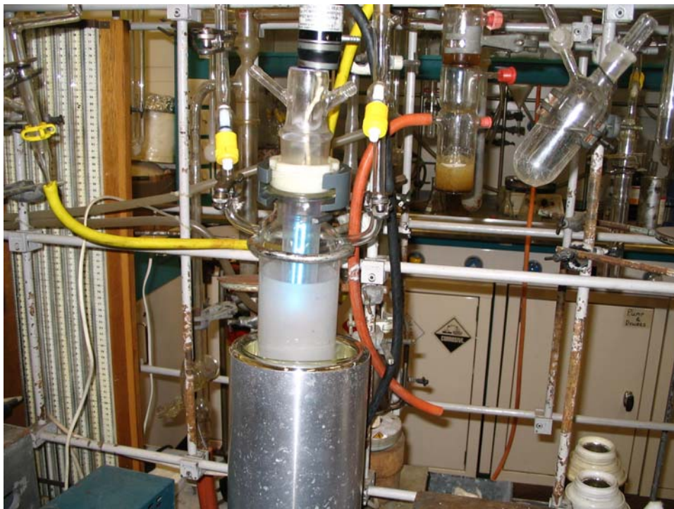
Fig. SM4.1 Reactor used in conjunction with a low pressure mercury arc lamp for photochemical studies on iron phosphides and meteoritic material. The frosted glass walls help the dispersion of solid powders on to the walls of the vessel to optimise irradiation area.
