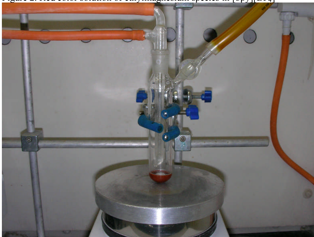
Figure 2. Red color solution of ethylmagnesium species in [bpy][BF 4 ]
