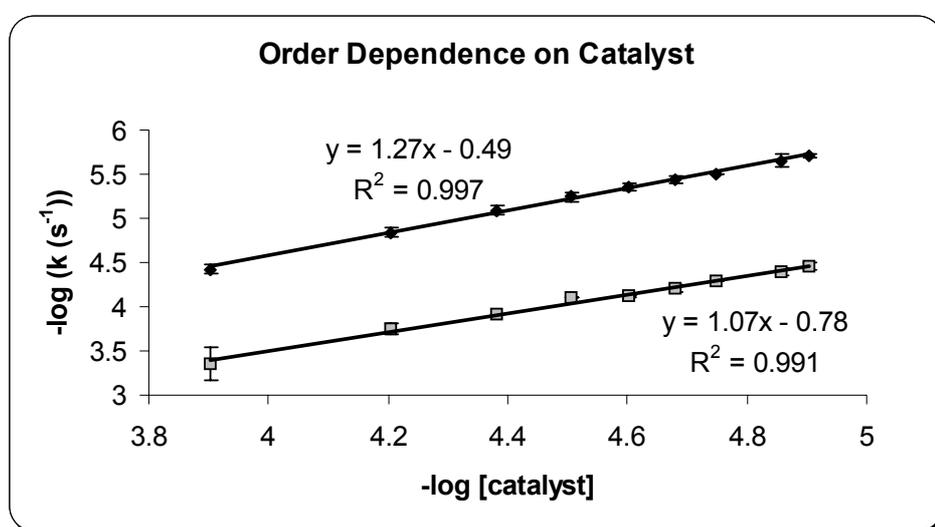
**Figure S1.** Determination of reaction order of catalysts  $^1\text{L}\cdot\text{Zn}_2$  (diamonds) and  $^2\text{L}\cdot\text{Zn}_2$  (squares) for the hydrolysis of PNPDP. Data are corrected for the non-catalyzed, background rate of hydrolysis.
