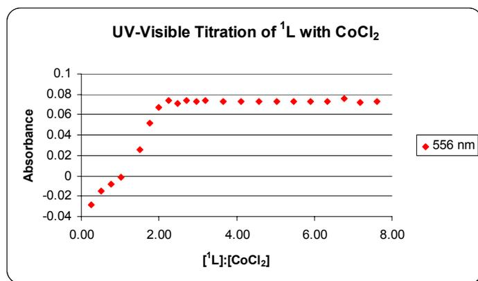
**Figure S6.** Absorption at 556 nm ( $\lambda_{\text{max}}$  for complex) for the titration of a 3.13 mM  $^1\text{L}$  solution (in DMF) with a DMF solution containing 3.13 mM  $^1\text{L}$  and 240 mM  $\text{CoCl}_2$ .
