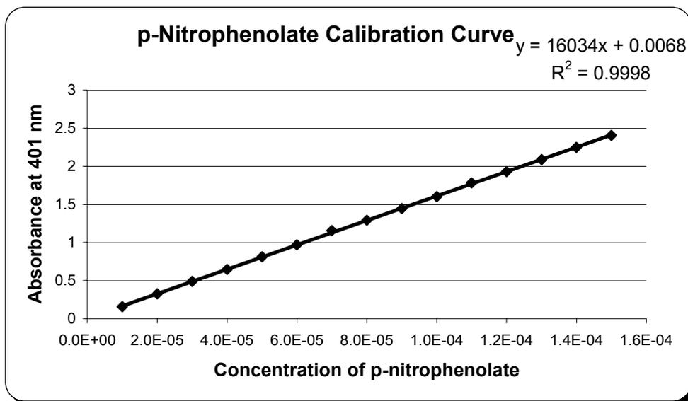
**Figure S2.** Determination of molar absorptivity at 401 nm for *p*-nitrophenolate ion using a Beer-Lambert plot. Experiment performed at ambient temperature using a 1.00 cm path length.
