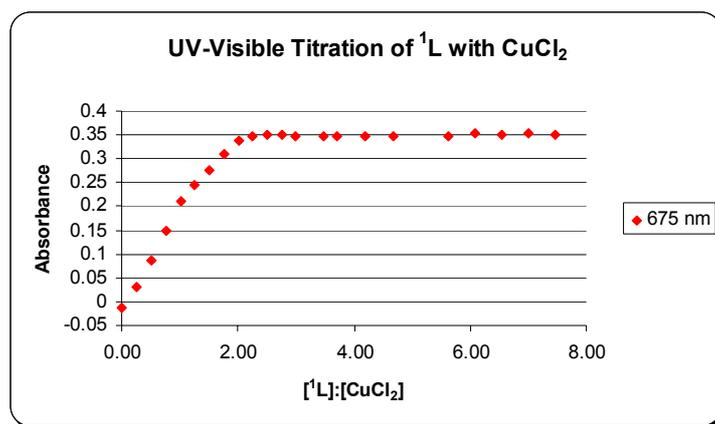
**Figure S5.** Absorption at 675 nm ( $\lambda_{\text{max}}$  for complex) for the titration of a 3.13 mM  $^1\text{L}$  solution (mixture of  $\text{H}_2\text{O}$ ,  $\text{EtOH}$ ,  $\text{DMF}$ ) with a solution containing 3.13 mM  $^1\text{L}$  and 399 mM  $\text{CuCl}_2$ .
