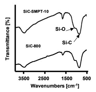
IR spectra of the mesoporous silicon carbide materials SiC-800 and SiC-SMPT-10. The Si-C bonds were detected at 830cm<sup>-1</sup> together with a minor presence Si-O species at 1040cm<sup>-1</sup>.
