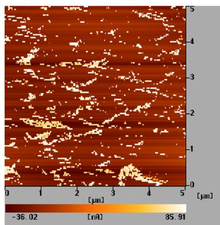
**Figure S2.** simultaneous current scanning image of the SnO<sub>2</sub> nanorod films
