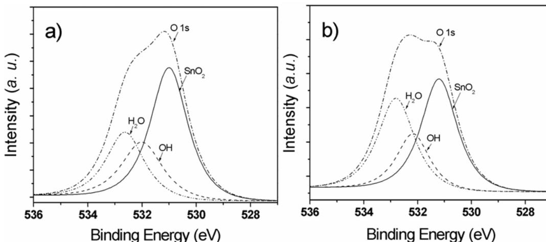
**Figure S1** O 1s spectra of the SnO<sub>2</sub> nanorod film a) before and b) after UV irradiation
