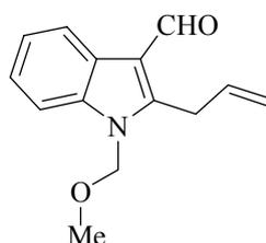
Prepared according to the typical procedure from 2-iodo-1-methoxymethyl-1H-indole-3-carbaldehyde (**1h**) (315 mg, 1.0 mmol), lithium dineophylcuprate **2** (1.2 mmol), and allyl bromide (360 mg, 3.0 mmol). Reaction time: 30 min at -78 °C. Purification by flash-chromatography (*n*-pentane/diethyl ether = 1/1) yielded the aldehyde **4l** as a light yellow solid (213 mg, 93%); mp 96 °C.
