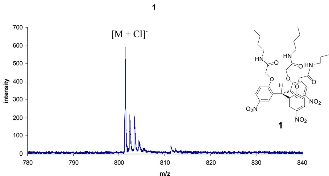
Figure 1: Negative mode ESI-MS for compound **1** in the absence of any TBA salts.
