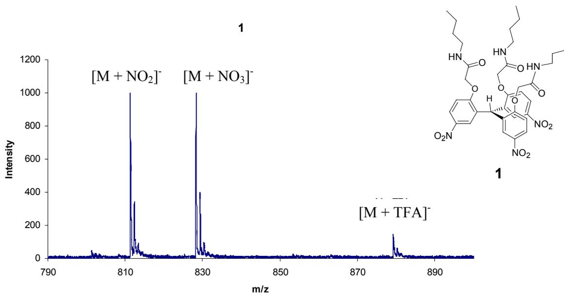
**Figure 2:** Negative-mode ESI-MS of **1** with TBANO<sub>3</sub> (1:1 mol%). We believe the significant [M + NO<sub>2</sub>]<sup>-</sup> peak originates from the reduction of the [M + NO<sub>3</sub>]<sup>-</sup> ion in the mass spectrometer in the (-)-mode ESI-MS.
