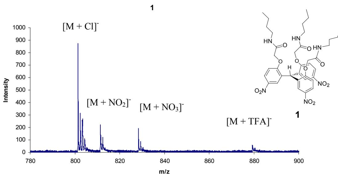
**Figure 3:** Negative mode ESI-MS of **1**. The mixture contained 1:1:1 TBACl: TBANO<sub>3</sub>: **1**.
