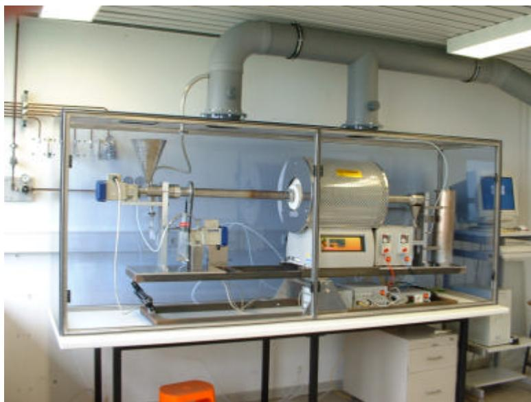
Pilot scale rotary kiln
