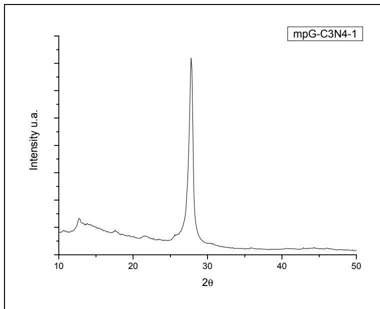
Small Angle X-Ray Diffraction of mpg-C<sub>3</sub>N<sub>4</sub>-1
