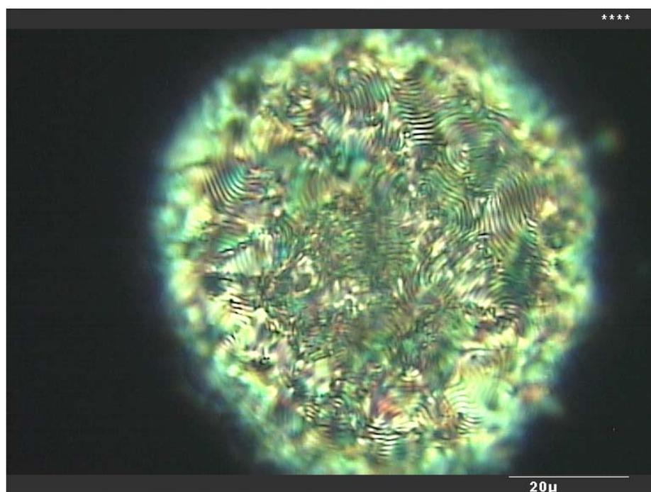
**Figure 3.** Texture of the chiral nematic phase displayed by **4** at room temperature.
