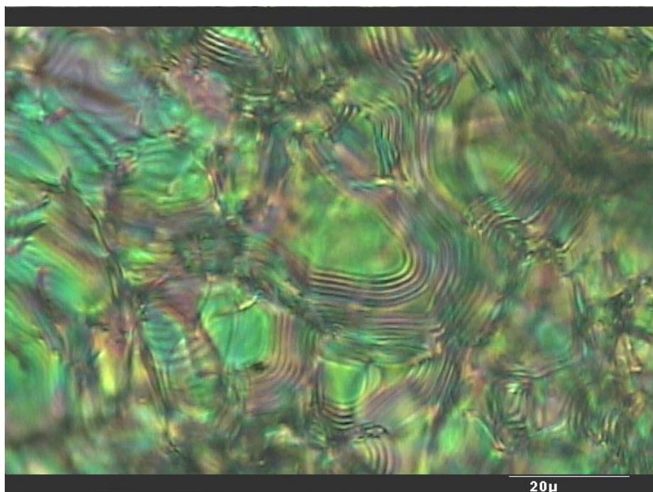
**Figure 1.** Texture of the chiral nematic phase displayed by **3** at room temperature.
