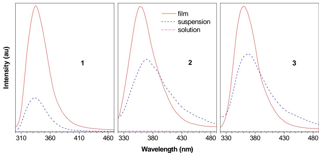
**Figure S2** PL spectra of **1**, **2** and **3** in dilute acetone solutions ( $20 \mu\text{M}$ ), as nanoparticle suspensions in the water/acetone mixtures with 90 vol % water contents, and in PMMA films (30 wt %).
