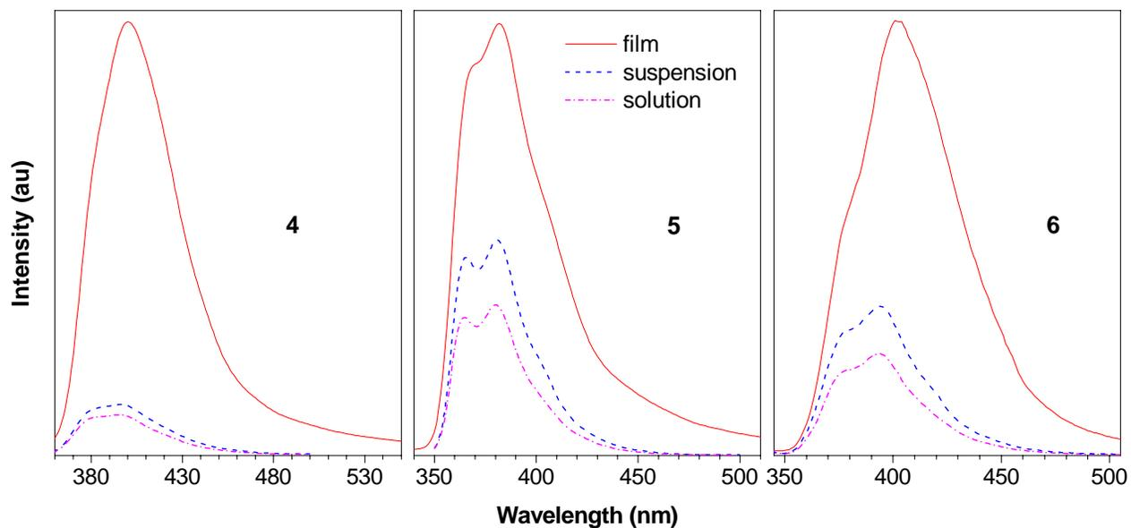
**Figure S4** PL spectra of **4**, **5** and **6** in dilute acetone solutions ( $20\ \mu\text{M}$ ), as nanoparticle suspensions in the water/acetone mixtures with 70 vol % water contents, and in PMMA films (30 wt %).
