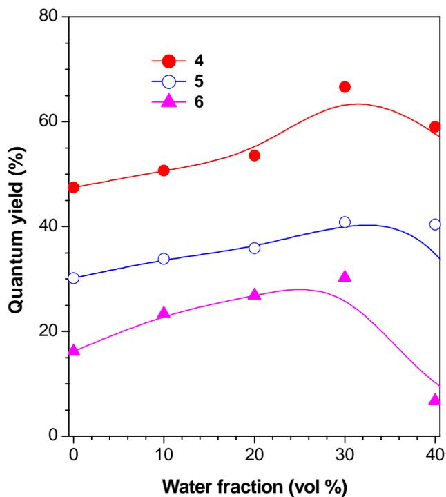
**Figure S5** Dependence of the fluorescence quantum yields of solutions of **4–6** ( $20\ \mu\text{M}$ ) on the water fractions in water/acetone mixtures.
