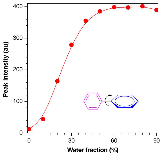
**Figure S1** Changes in the PL peak intensity of biphenyl in the water/DMF mixtures with different water contents. Biphenyl concentration: 20  $\mu\text{M}$ . Excitation wavelength: 263 nm.
