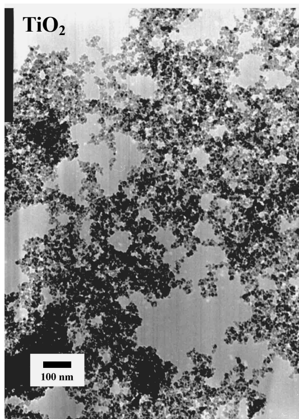
Figure S2 TEM images of \text{TiO}_2 (left) and \text{ZrO}_2 (right) nanoparticles prepared from molten salt method. The average particle size is 10.1 nm and 4.6 nm for \text{TiO}_2 and \text{ZrO}_2 , respectively.
