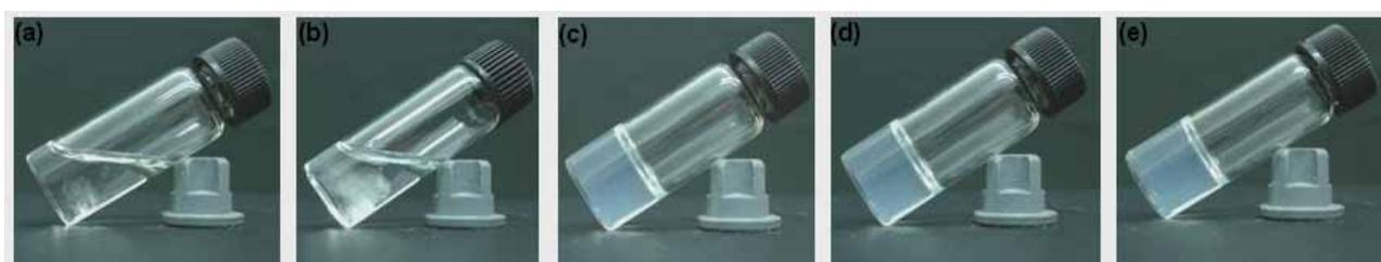
**Fig. S10.** Pictures of HPMA-1 in DMF at (a)  $1.0 \text{ mg mL}^{-1}$ ; (b)  $2.0 \text{ mg mL}^{-1}$ ; (c)  $2.5 \text{ mg mL}^{-1}$ ; (d)  $20 \text{ mg mL}^{-1}$ ; (e)  $40 \text{ mg mL}^{-1}$ . The flocs are visible in the flasks below the CGC (see a and b). The immobile gels are formed at or above the CGC (see c, d and e).
