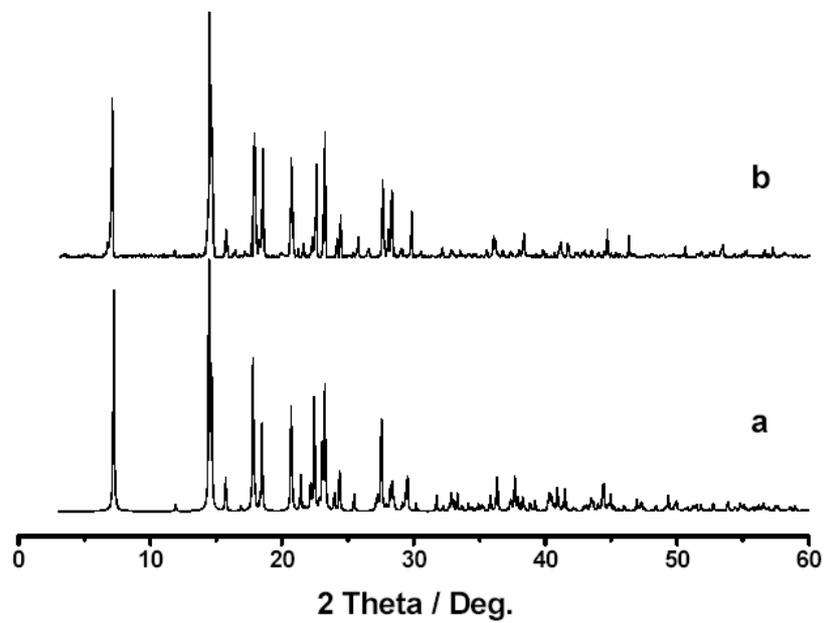
**SI-1** PXRD patterns of **1**: (a) the simulated one from single crystal data and (b) the original one at room temperature.
