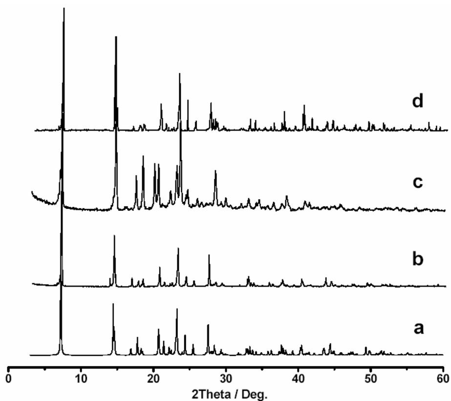
**SI-2** PXRD patterns of **2**: (a) the simulated one from single crystal data, (b) the original one at room temperature, (c) the dehydrated one *via* heating to 270 °C, and (d) the re-hydrated one.
