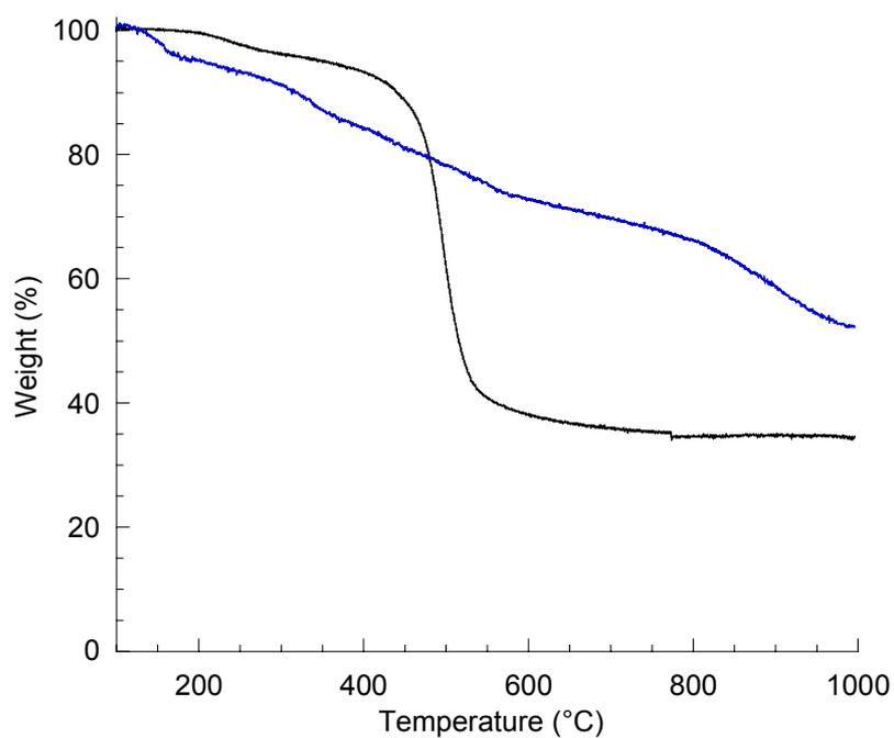
**Fig. S1** Thermogravimetric analysis of the SWNT-H<sub>2</sub>Pc nanoconjugate **1** (blue) and of the phthalocyanine **4** (black).
