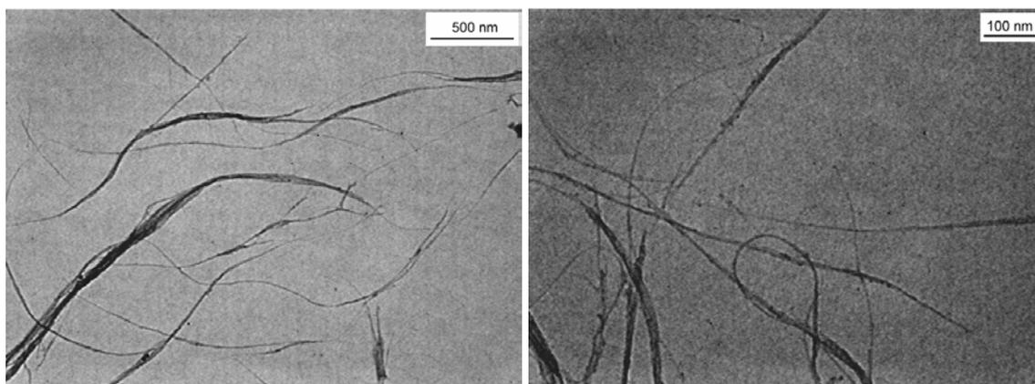
**Fig. S2** TEM pictures of SWNT-H<sub>2</sub>Pc nanoconjugate **1**. Left image: general view showing large aspect ratio material. Right image: higher magnification picture showing the quasi-absence of metal catalyst nanoparticles on the nanotubes.
