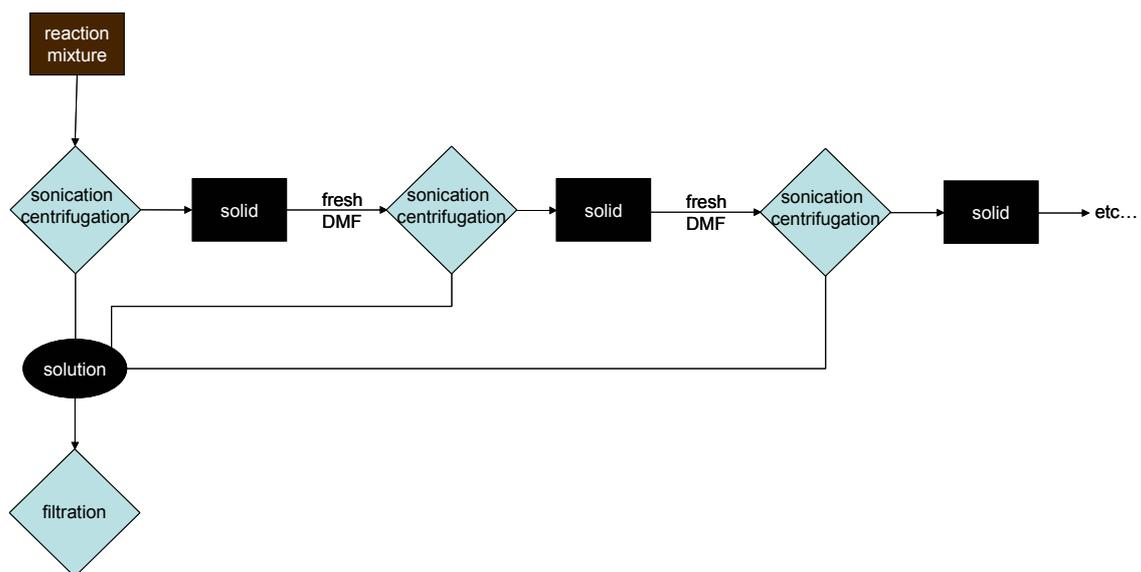
**Fig. S3** Schematic representation of the work up procedure for the synthesis of f-SWNT
