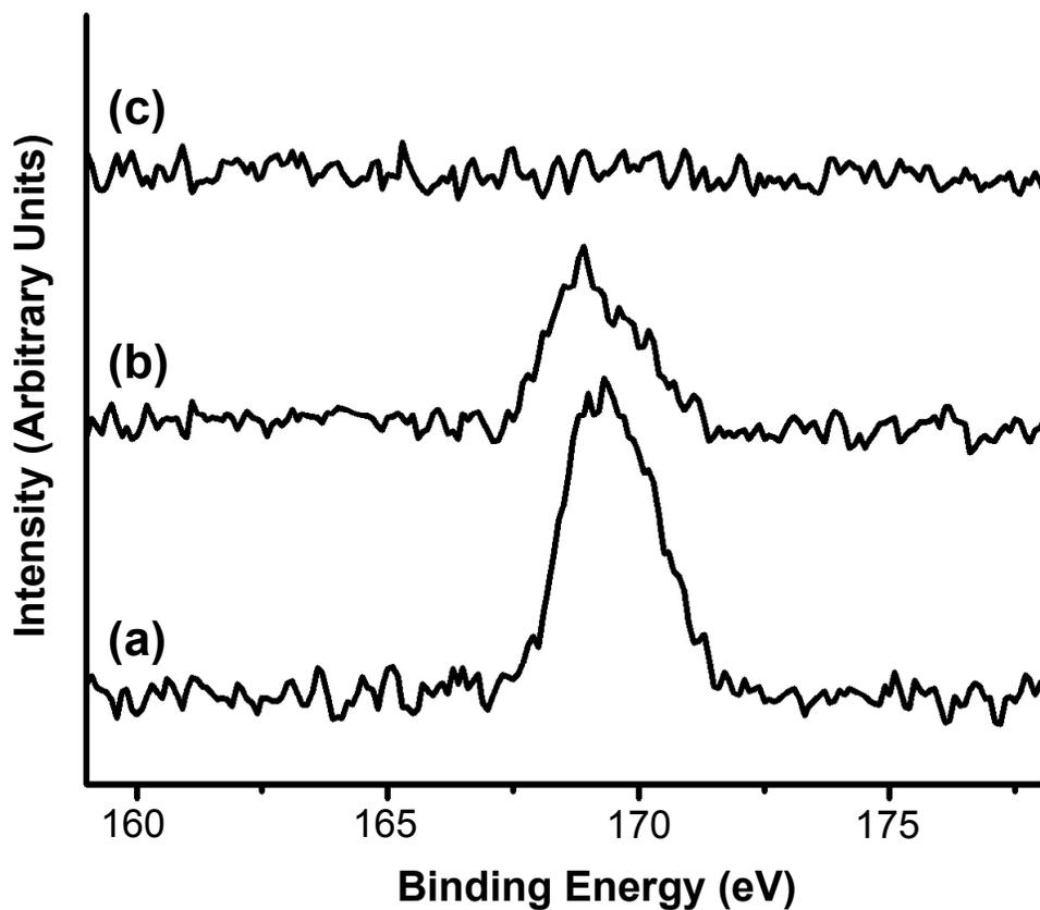
**Figure 3S.** Sulfur 2p X-ray photoelectron spectra for SnO<sub>2</sub> films deposited with 2 w % SDS; (a) as-deposited after 30 s of rinsing, (b) after 3 hours of soaking in DI water, and (c) after 12 hours of soaking in DI water. Note the disappearance of the sulfur peak in sample (c) due to removal of SDS.
