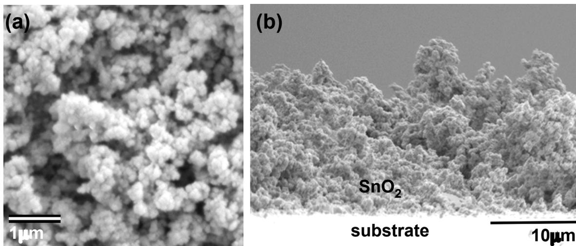
**Figure 1S.** SEM images of (a) top and (b) side view of mesoporous  $\text{SnO}_2$  Films.
