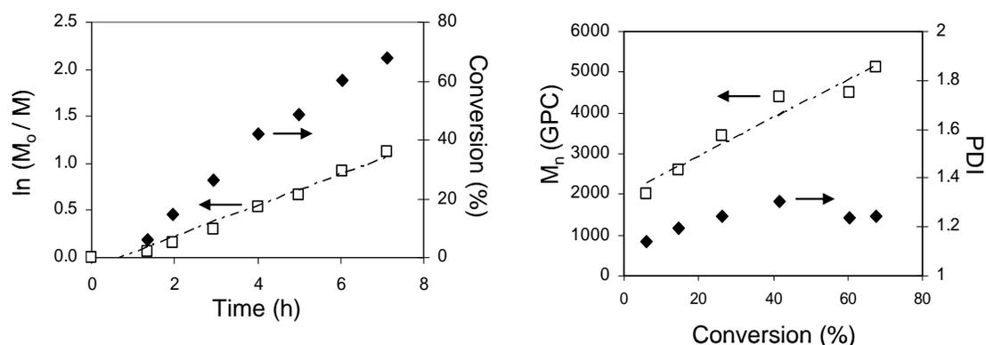
**Figure S1.** (a) Kinetic plot and (b)  $M_n$  and PDI with respect conversion for RAFT polymerization of DEPMA (100:5:1 of DEPMA:CDB:AIBN) at 70 °C in DMF.
