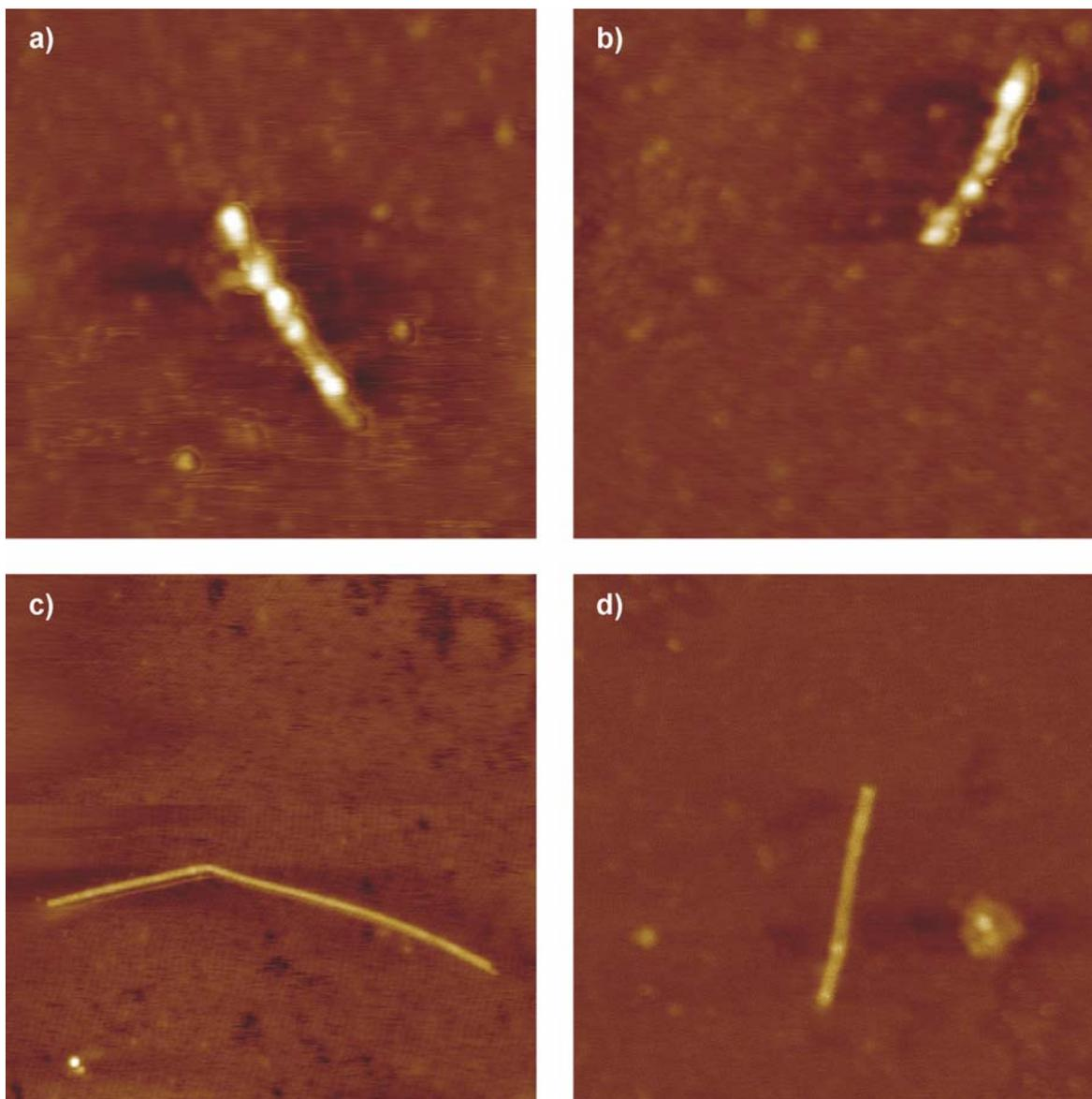
**Figure S1.** AFM of samples treated with thionyl chloride and cysteamine after exposure of gold colloids (a, b) sample C', 400x400 nm; (c) blank experiment conducted on sample A', 750x750 nm; (d) blank experiment conducted on sample C, 400x400 nm. In all images  $z$  scale is 0-5 nm. Gold nanoparticles (large bright dots) can clearly be seen along SWNT walls in sample C' (a&b). In contrast, no gold nanoparticles are present along the SWNT walls in the blank experiments (c&d).
