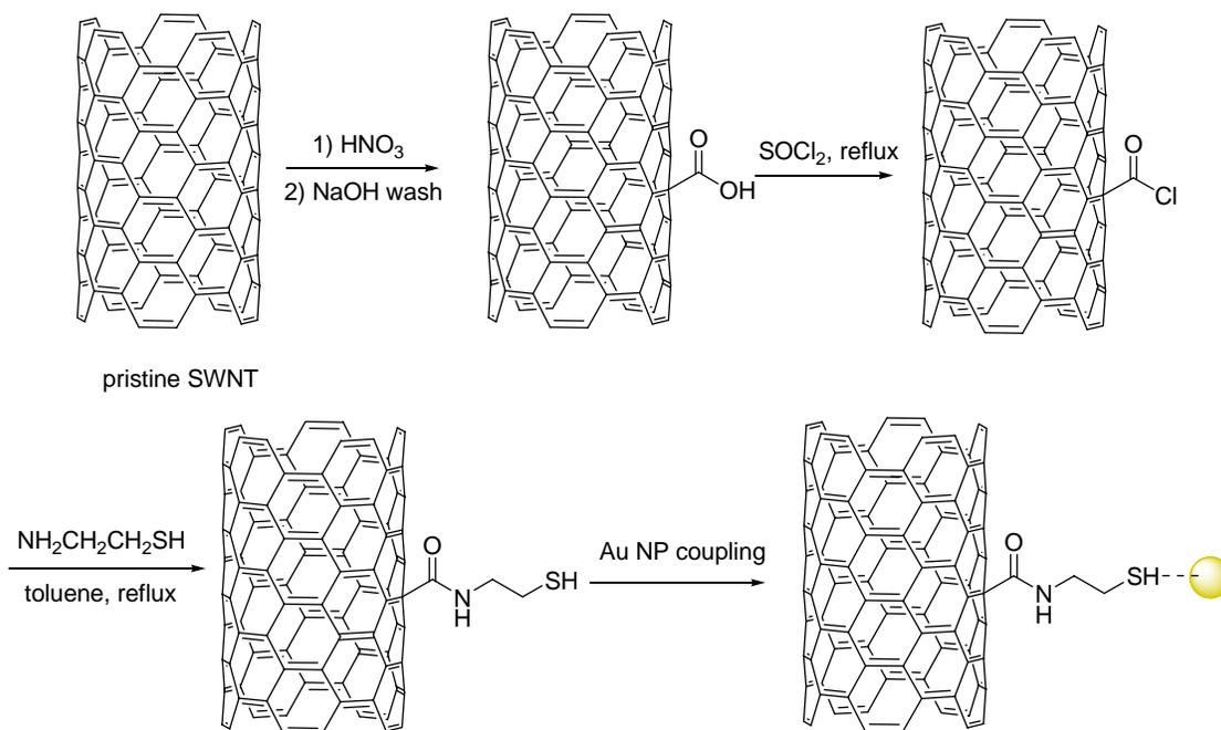
**Scheme S2.** Cysteamine coupling to steam purified, acid treated and base washed SWNTs (Sample C').
