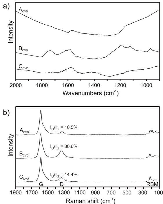
**Figure S2.** a) FTIR and b) Raman spectra of as-received CVD SWNTs (sample A<sub>CVD</sub>), after acid treatment (sample B<sub>CVD</sub>) and base wash (sample C<sub>CVD</sub>).
