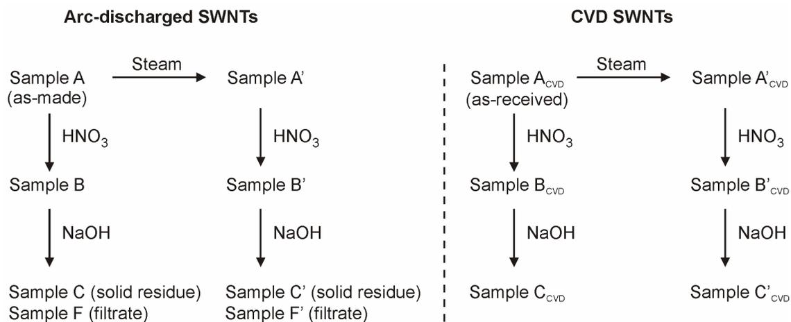
**Scheme S1.** Schematic representation of the treatments done on arc-discharged and CVD SWNTs. For ease of comparison between samples, steam treated SWNTs are indicated by the superscript [<sup>'</sup>] and CVD SWNTs by the subscript [<sub>CVD</sub>]. All the treatments are followed by washing with distilled water.
