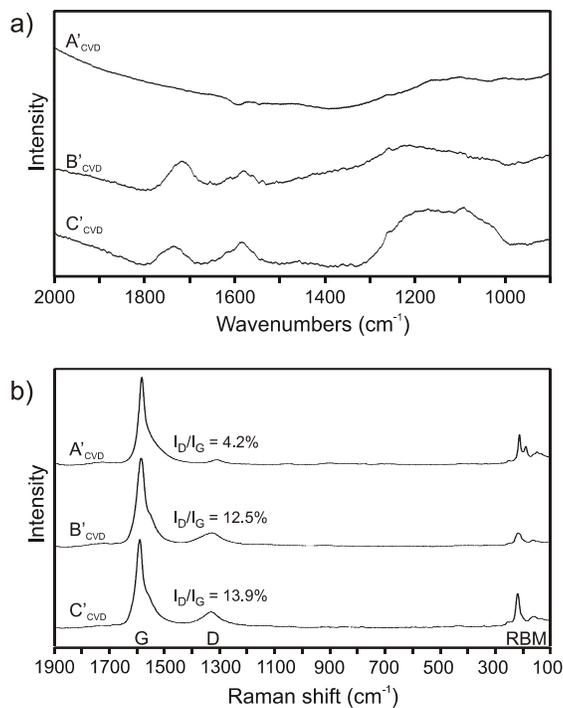
**Figure S3.** a) FTIR and b) Raman spectra of steam purified CVD SWNTs (sample A'<sub>CVD</sub>), after acid treatment (sample B'<sub>CVD</sub>) and base wash (sample C'<sub>CVD</sub>).
