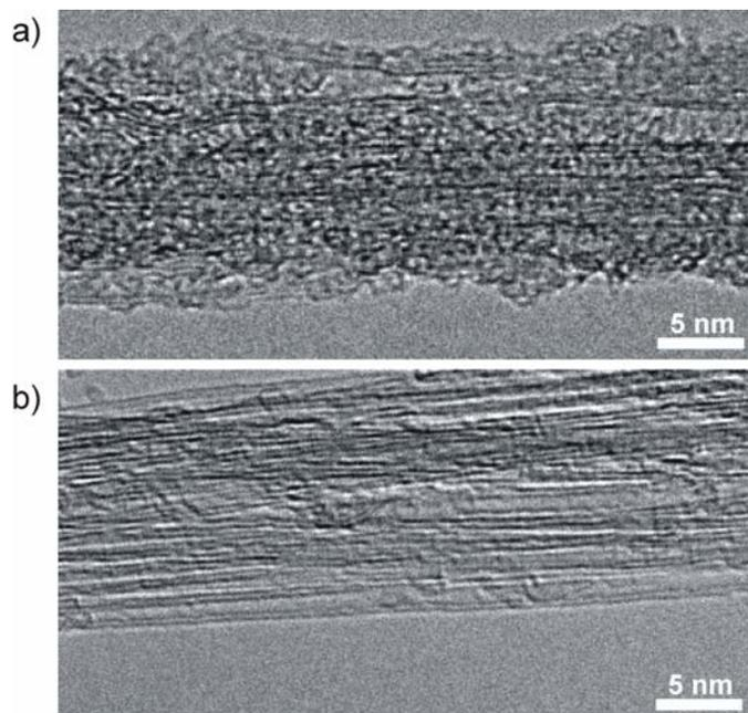
**Figure S4.** HRTEM image of a) as-received CVD SWNTs after nitric acid treatment (sample B<sub>CVD</sub>) and b) steam purified CVD SWNTs after nitric acid treatment (sample B'<sub>CVD</sub>). A much larger degree of amorphous coating (oxidation debris) can be seen in image (a) compared to (b).
