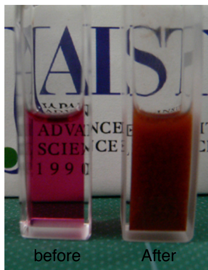
Fig S1. Pictures of 0.35 mmol dm -3 H 2 DBuPP solutions (acetonitrile/toluene = 9/1, v/v) before and after sonication.
