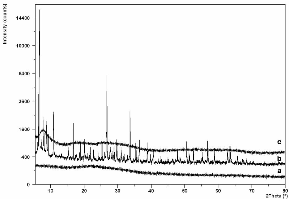
Fig. S2. Powder X-ray diffraction patterns of (a) core-crosslinked PB-P2VP polymeric nanorod template (b) pure  $\text{H}_4[\text{SiMo}_{12}\text{O}_{40}]$  and (c) POM-1
