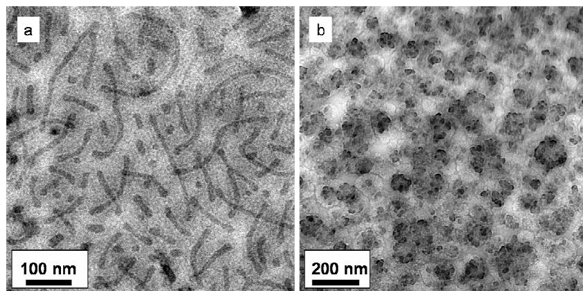
Fig. S1. Cryo-TEM images of the (a) 1 wt% of  $\text{PB}_{80}\text{-P2VP}_{20}$  (64,900 g/mol) in THF wormlike micelles without core crosslinking, (b) 1 wt% of  $\text{PB}_{80}\text{-P2VP}_{20}$  (64,900 g/mol) in THF acidified with 2M HCl.
