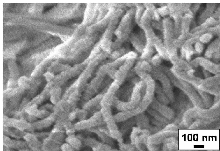
Fig. S3 SEM image of the  $[\text{PMo}_{12}\text{O}_{40}]^{3-}$  keggin POM grafted over core-crosslinked PB-P2VP worm-like polymer template
