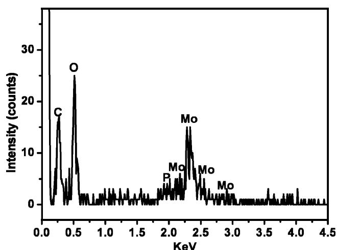
Fig. S4 EDX spectrum of the  $[\text{PMo}_{12}\text{O}_{40}]^{3-}$  keggin POM grafted over core-crosslinked PB-P2VP worm-like polymer template
