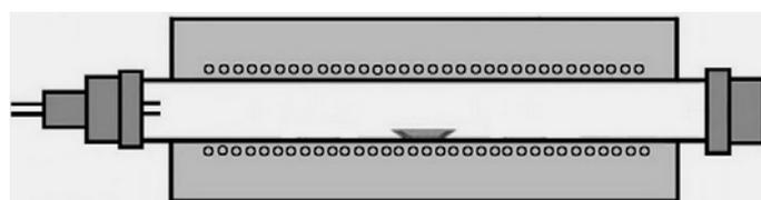
**Figure S0.** The sketch map of the tube furnace used for thermolysis.
