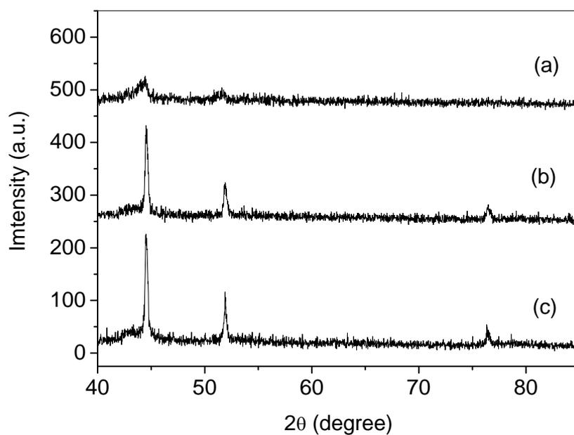
**Figure S5.** XRD patterns of the synthesized MWCNTs by thermolysis of the Ni-MOF in the one-end closed horizontal tube furnace at 500 °C for (a) 5 h, (b) 10 h, (c) 15 h, and (d) 20 h.
