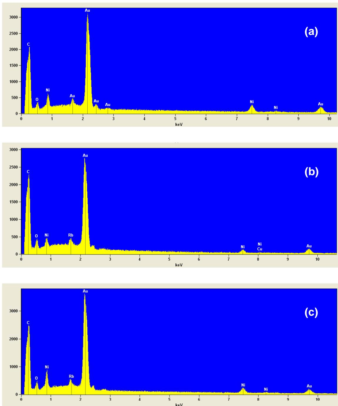
**Figure S7.** FE-SEM image and EDX of the remained Ni particles after thermolysis of the Ni-MOF in the one-end closed horizontal tube furnace at 500 °C for 20 h.
