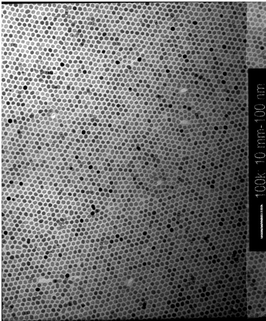
Figure S1a. TEM image of  $\text{In}_2\text{O}_3$  core nanocrystals.
