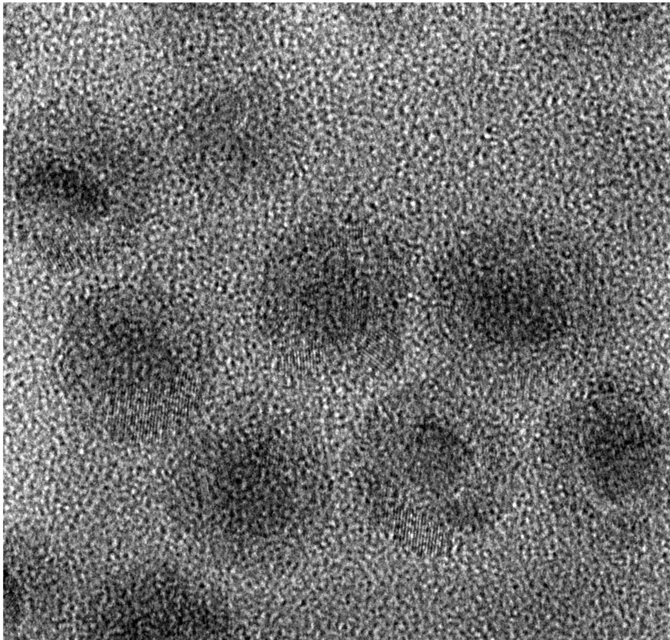
Figure S1c. High-resolution TEM image of  $\text{In}_2\text{O}_3\text{-In}_2\text{S}_3$  nanoparticles.
