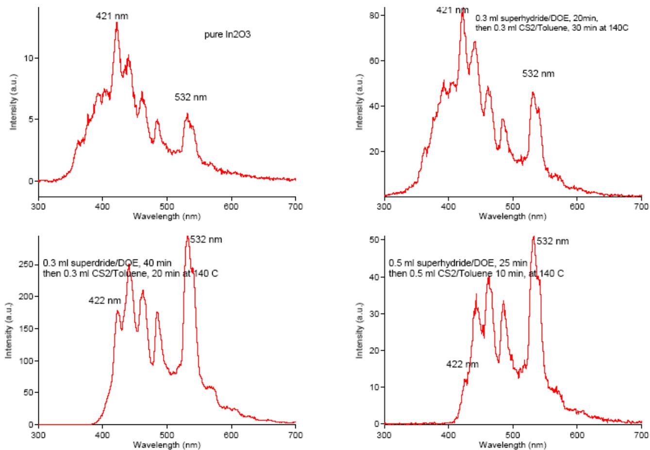
Figure S2. Photoluminescence spectra recorded with various reaction conditions, showing that the reduction step is more important than the sulfidization step for the formation of In<sub>2</sub>S<sub>3</sub> shell.
