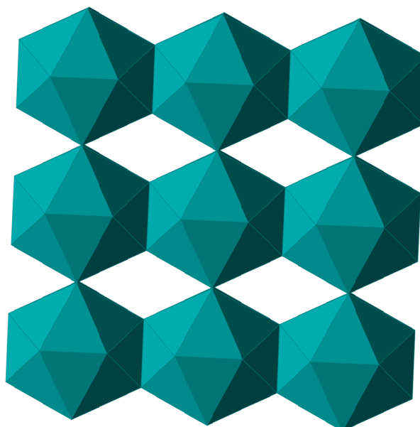
Figure S2. Representation of one plane of the \text{Cs}_8\text{Sn}_{46} structure showing four of the six edge-sharing \text{Cs}_{12} icosahedra connected to the central one that are responsible for a primitive cubic packing.
