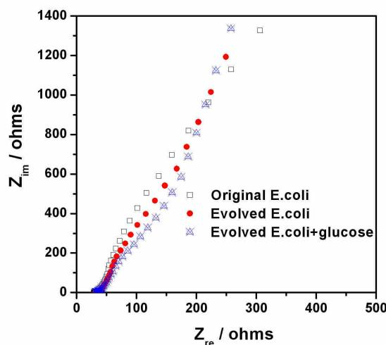
Electrochemical impedance spectra measurements were performed over a frequency range of 0.5Hz to 100 kHz at open circuit potential with a perturbation signal of 10 mV. The Nyquist plots
