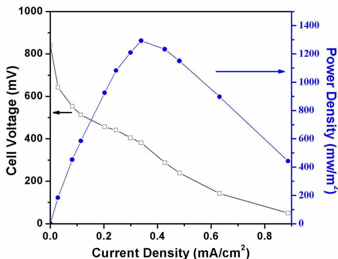
The power output of the mediator-less MFC with evolved E. coli cells as biocatalyst were examined with various resistances. The open-circuit potential is 830 mV and the maximum power density is 1300 mW/m<sup>2</sup>, corresponding to a current density of 3390 mA/m<sup>2</sup> at a cell potential of 340 mV.
