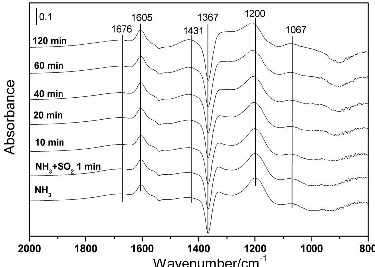
**Fig.9** *in situ* DRIFTS spectra of adsorbed species on  $\text{Fe}_x\text{TiO}_y$  after  $\text{SO}_2$  addition in a flow of  $\text{NH}_3$  at  $200\text{ }^\circ\text{C}$
