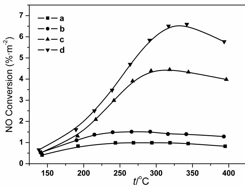
**Fig.6** Specific activity per surface area of catalysts under different calcination temperature for 6 h:
