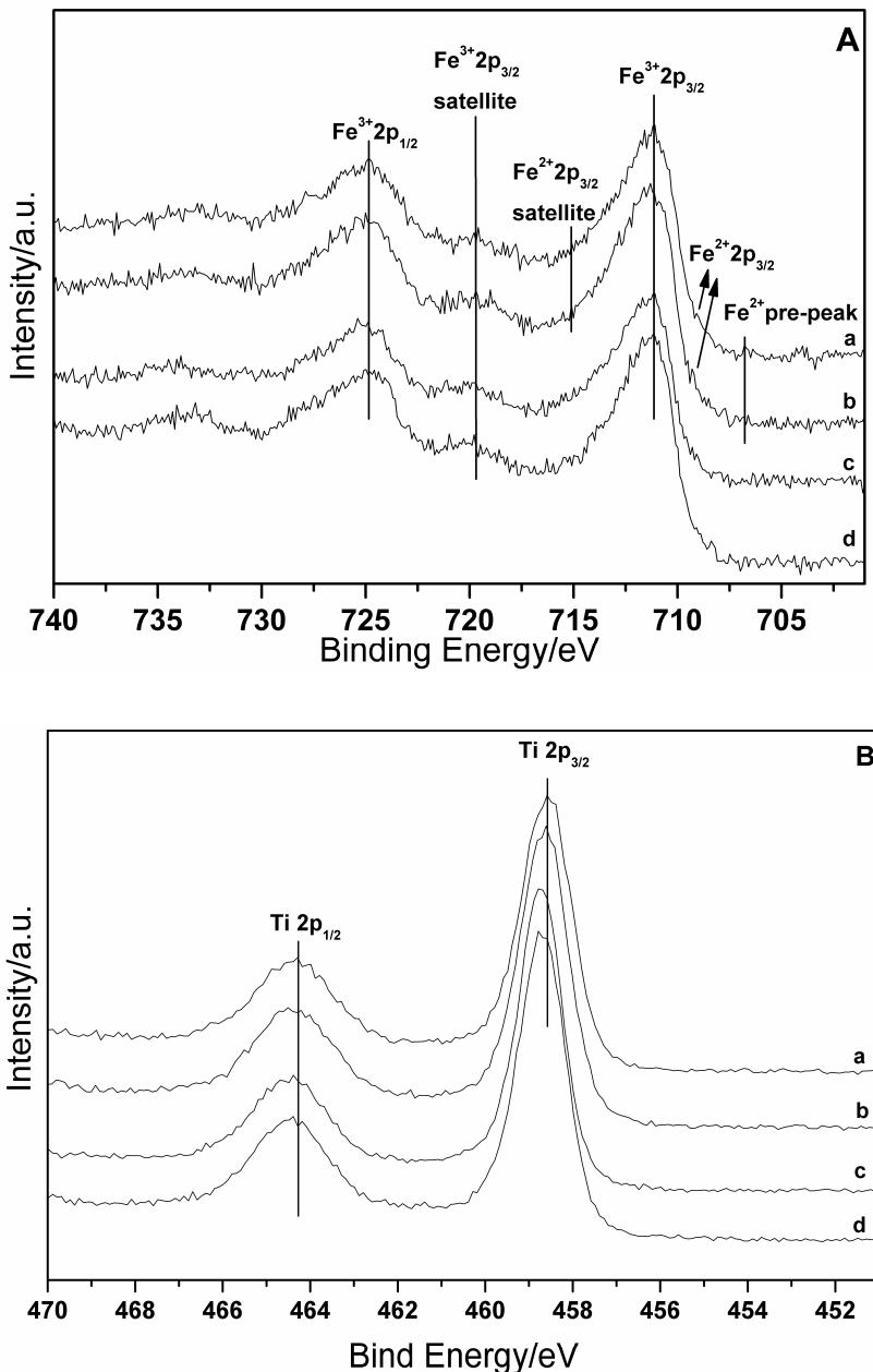
**Fig. 7** XPS results of catalysts under different calcination temperature for 6 h:
