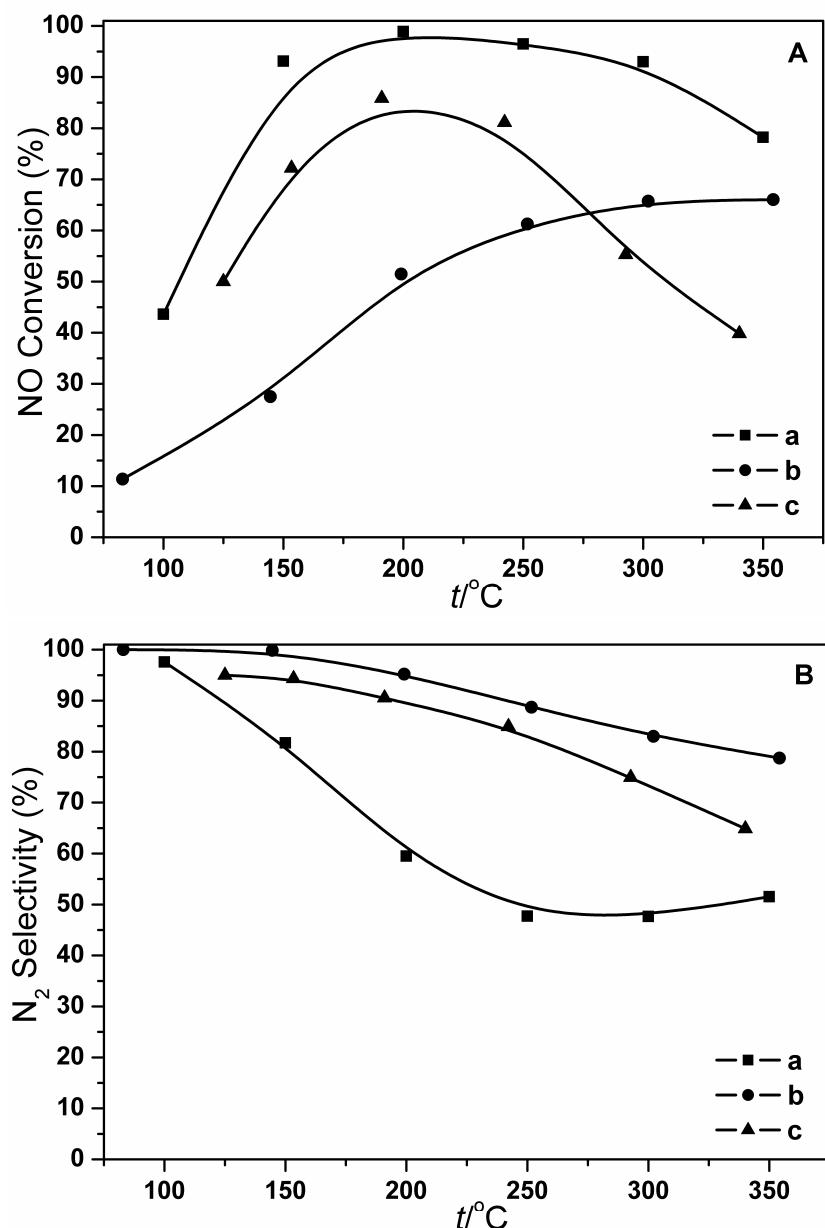
**Fig.3** NO conversion (A) and N<sub>2</sub> selectivity (B) over (a) 10wt% $MnO_x/TiO_2$ ; (b)  $MnO_x/TiO_2$  (Mn:Ti=1 in molar ratio); (c)  $CuO_x/TiO_2$  (Cu:Ti=1 in molar ratio).
