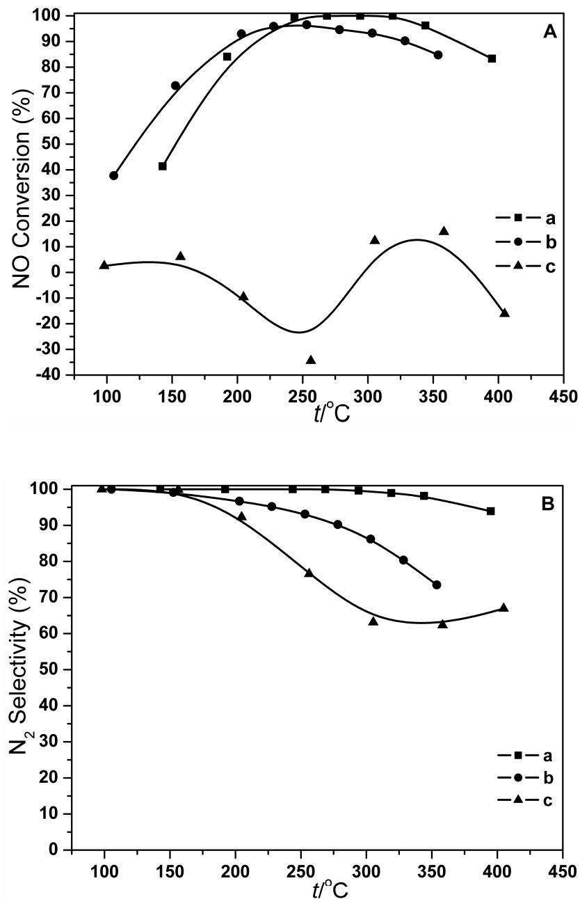
**Fig.2** NO conversion (A) and  $\text{N}_2$  selectivity (B) over (a)  $\text{Fe}_x\text{TiO}_y$ ; (b)  $\text{Mn}_x\text{TiO}_y$ ; (c)  $\text{Cu}_x\text{TiO}_y$ .
