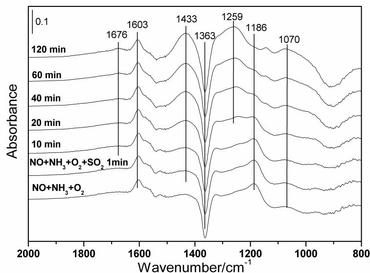
**Fig.10** *in situ* DRIFTS spectra of adsorbed species on  $\text{Fe}_x\text{TiO}_y$  after  $\text{SO}_2$  addition in a flow of  $\text{NO}+\text{NH}_3+\text{O}_2$  at  $200\text{ }^\circ\text{C}$
