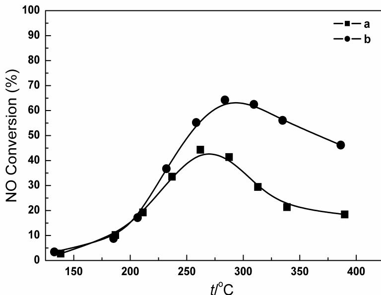
**Fig.4** NO conversion over (a)  $\text{Fe}_2\text{O}_3+\text{TiO}_2$  mixed; (b)  $\text{Fe}_2\text{O}_3+\text{TiO}_2$  mixed and calcined.
