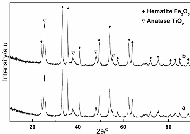
**Fig.5** XRD patterns of (a)  $\text{Fe}_2\text{O}_3+\text{TiO}_2$  mixed; (b)  $\text{Fe}_2\text{O}_3+\text{TiO}_2$  mixed and calcined.
