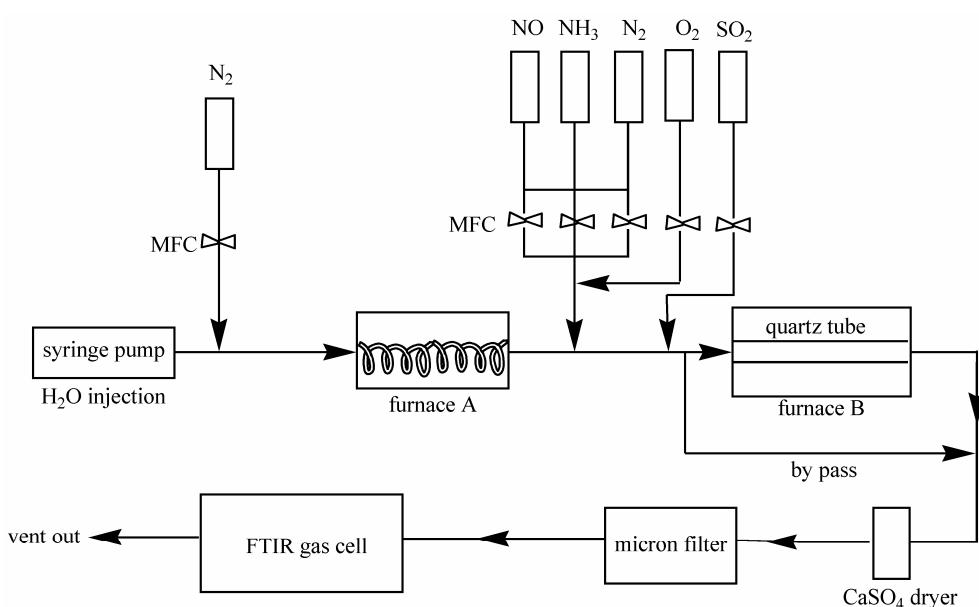
**Fig.1** NH<sub>3</sub>-SCR activity test system: Furnace A for water gasification; Furnace B for SCR reaction
