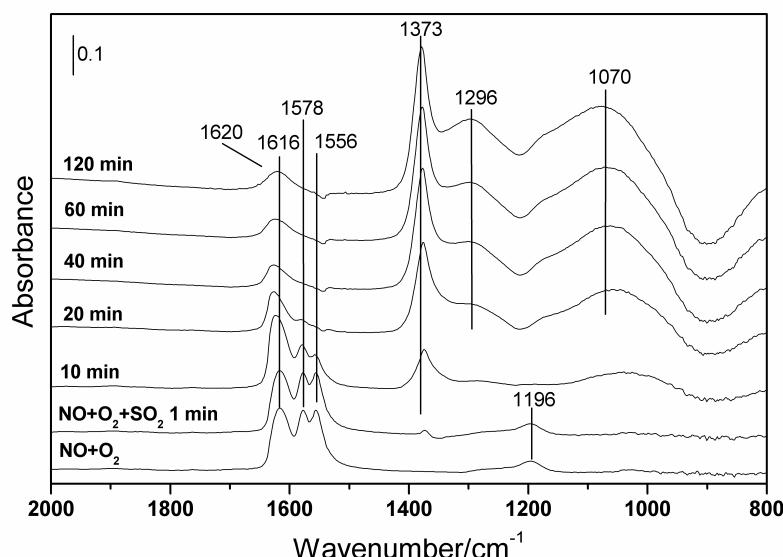
**Fig.8** *in situ* DRIFTS spectra of adsorbed species on Fe<sub>x</sub>TiO<sub>y</sub> after SO<sub>2</sub> addition in a flow of NO+O<sub>2</sub> at 200 °C.
