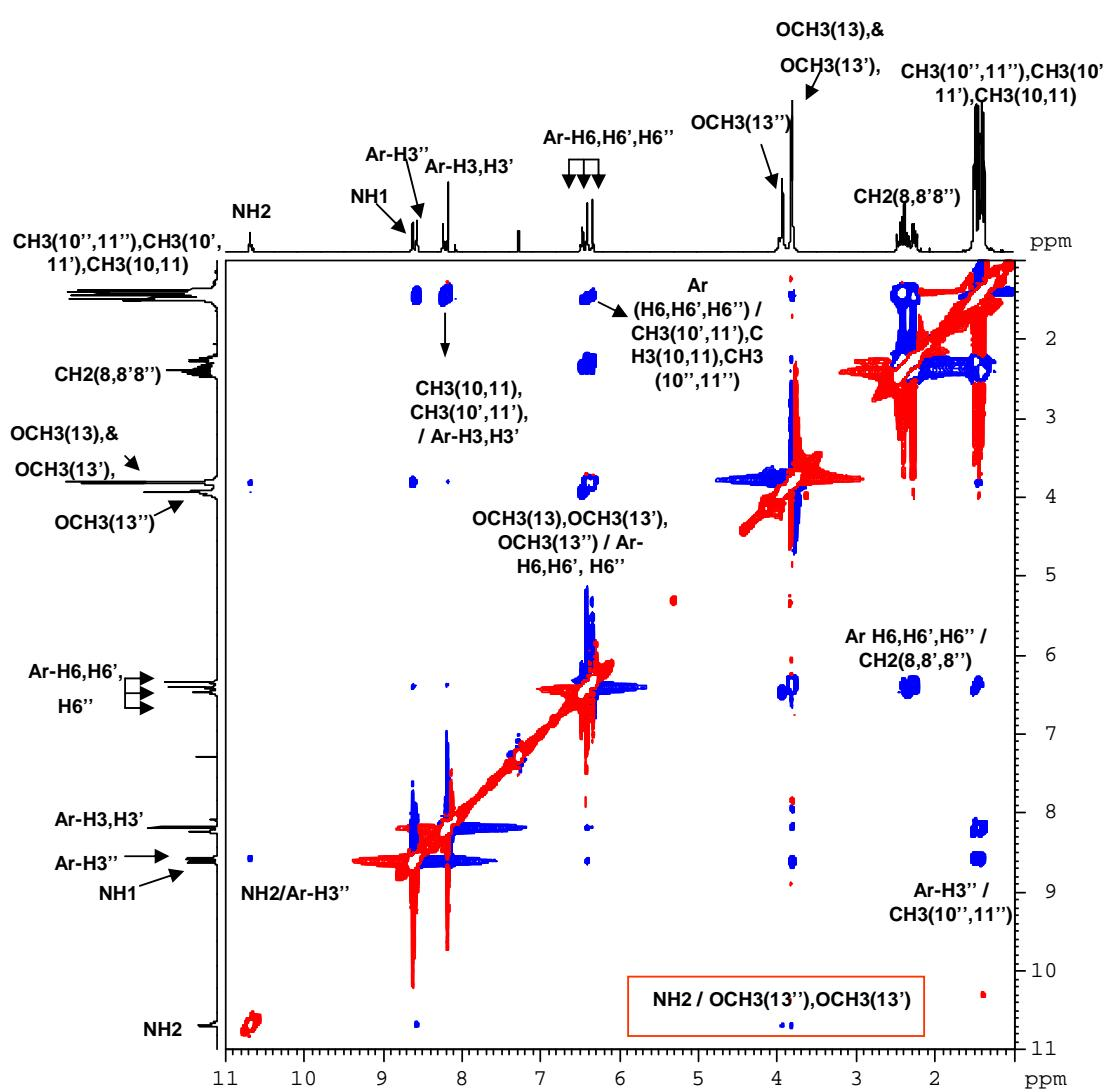
**Figure 3.** 2D ROESY spectrum of the oligomer **2** ( $\text{CDCl}_3$ , 400 MHz). Note: The bifurcated H-bonding interaction (NH vs OMe) has been highlighted with red border.
