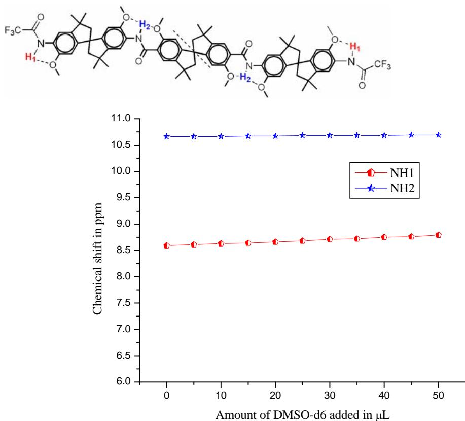
**Figure 1.** Molecular structure of foldamer **2** (*top*) and its DMSO-*d*<sub>6</sub> titration graph (*bottom*). The initial concentration of the sample in CDCl<sub>3</sub> was 5 mmol, and the total amount of [D6]DMSO used was 11 % of the total volume.
