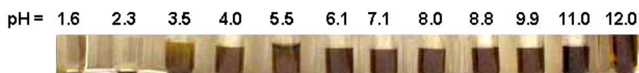
Figure S2. Behavior of the HMBP coated nanoparticles solution as function of pH. The initial conditions are at pH 7.1 and iron concentration of 4 \times 10^{-3} \text{ mol.L}^{-1} %. The suspension pH is then adjusted with sodium hydroxide (NaOH) or acidic (HCl) solutions. Below pH 4.0, a macroscopic phase separation is observed through the apparition of a black precipitate (bottom phase).
