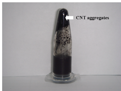
Fig. S3. A photograph of Pluronic F-127 coated CNTs after incubation in 10% serum-containing medium for 3 days.
