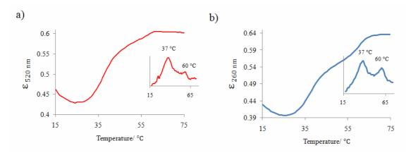
UV-Vis triplex melting curves at a) 520 nm b) 260 nm. First derivatives and melting temperatures shown in insets.
