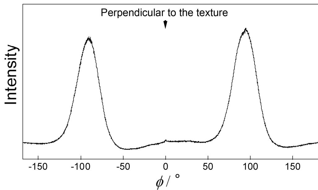
**Figure S3** In-plane  $\phi$  scanning profile of mesostructured film prepared by hydrothermal deposition method recorded for the diffraction peak at  $2\theta\chi = 1.3^\circ$ .
