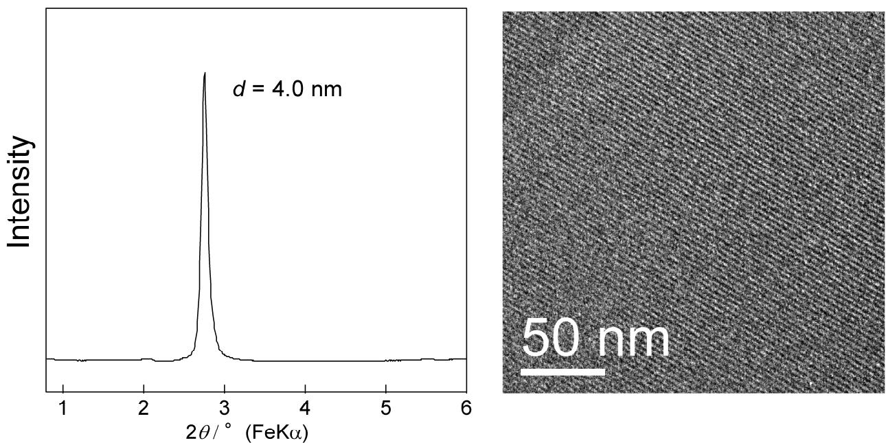
**Figure S2.** The conventional  $\theta$ - $2\theta$  scanning XRD profile and TEM image of mesoporous silica film prepared by EISA method on a freshly cleaved mica surface.
