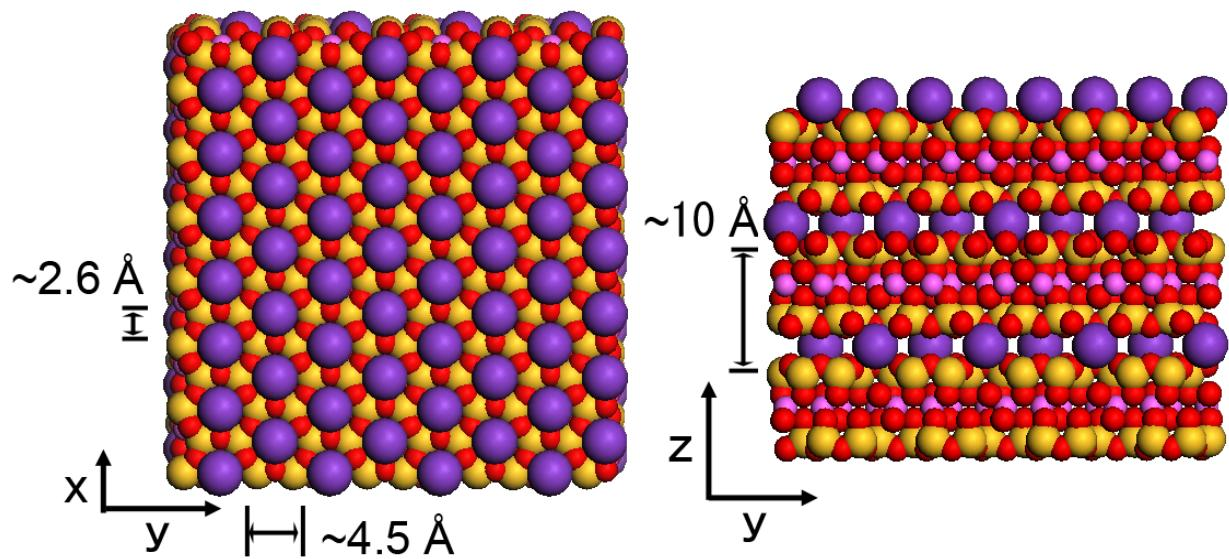
**Figure S1.** Crystal structure of mica created by using Material Studio software. Color spheres; red = O, yellow = Si, pink = Al, purple = K. A quarter of  $\text{SiO}_4$  are replaced with  $\text{AlO}_4$  tetrahedra.
