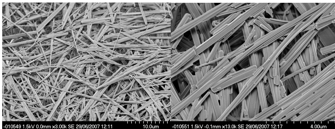
Figure S1. SEM images of compound 1 n = 2 xerogel formed from an acetonitrile gel. Note how the gel fibres are rod-shaped and show no indication of the chirality of the gelator.
