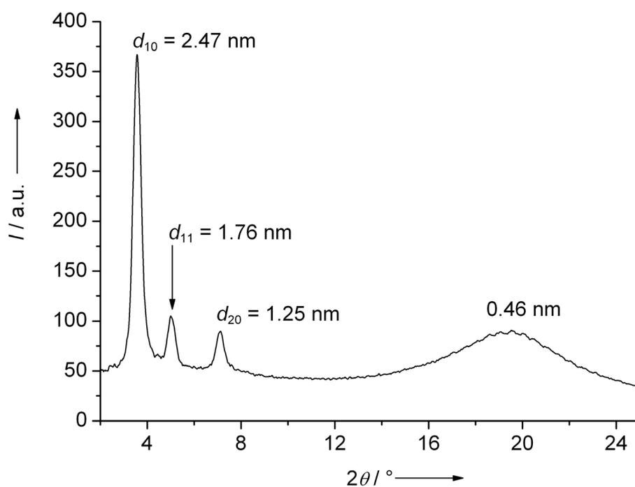
**Figure S1.** Powder diffraction pattern of the Col<sub>squ</sub>-phase of **A1** at  $T = 55$  °C with  $d$  values for the observed reflections and for the maximum of the diffuse outer scattering.
