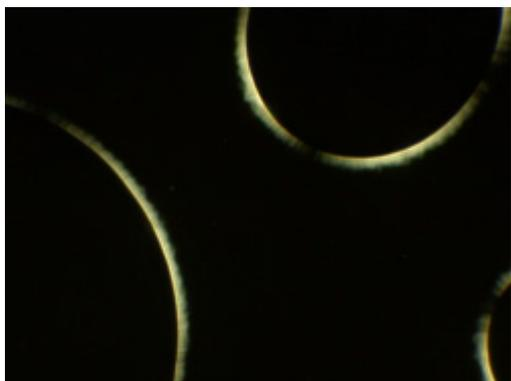
**Figure S6.** Texture of the  $Lam_{Iso}$  phase of compound **C4** at  $T = 140$  °C (birefringence is seen only around the air bubbles, the dark area outside the air bubbles is the homotropically aligned  $Lam_{Iso}$  phase).
