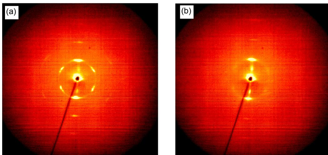
**Figure S4.** X-ray diffraction patterns (small angle region) obtained from mesophases of the surface-aligned sample **C3**: (a)  $Col_{hex}/p6mm$ -phase at  $T = 81$  °C; (b)  $Lam_{Iso}$ -phase at  $T = 113$  °C.
