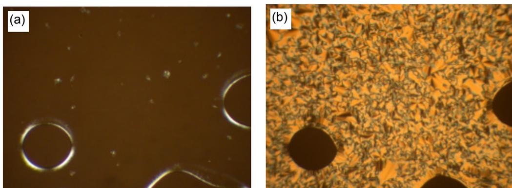
**Figure S5.** Texture of compound **C3** in the (a)  $Lam_{Iso}$  phase at  $T = 113$  °C and (b)  $Col_{hex}/p6mm$  phase at  $T = 80$  °C.
