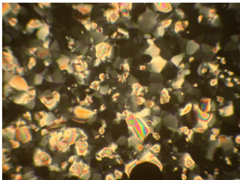
**Figure S3:** Texture of the  $\text{Col}_{\text{hex}}/p6mm$  phase of compound **C2** at  $T = 80$  °C.
