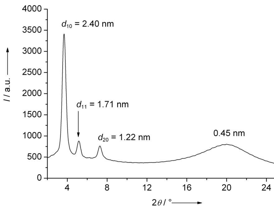
**Figure S2.** Powder diffraction pattern of the  $\text{Col}_{\text{squ}}$ -phase of **B2** at  $T = 28$  °C with  $d$  values for the observed reflections and for the maximum of the diffuse outer scattering.
