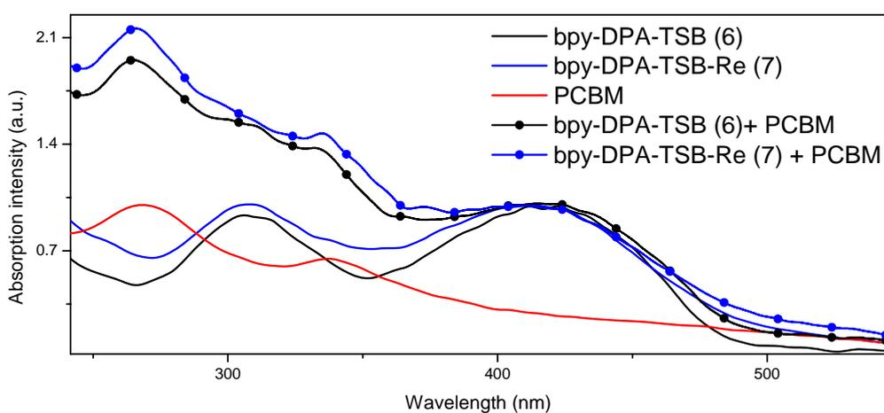
**Fig. S4.** The thin film absorption spectra of bpy-DPA-TSB (**6**), bpy-DPA-TSB-Re (**7**), PCBM and their blends with PCBM (1:1, w/w), all films were prepared by spin-coating using  $5 \text{ mg mL}^{-1}$  solution.
