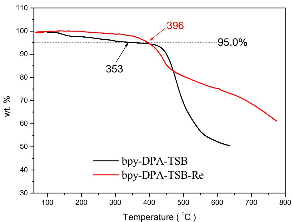
**Fig. S6.** TGA of of bpy-DPA-TSB (6) and bpy-DPA-TSB-Re (7).
