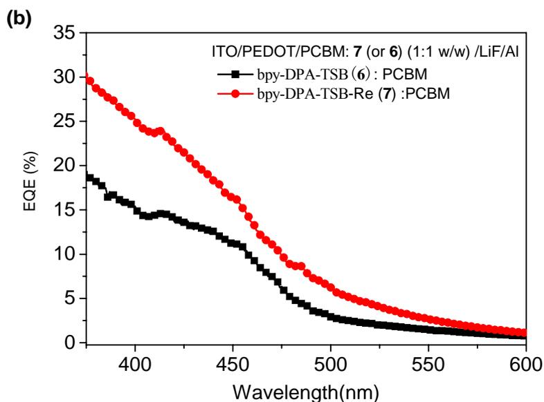
**Fig. S7.** a) Comparison of the external quantum efficiency (EQE) spectra of photovoltaic devices based on bpy-DPA-TSB (6) and bpy-DPA-TSB-Re (7); b) Comparison of the EQE spectra of photovoltaic devices based on bpy-DPA-TSB (6) : PCBM (1:1, w/w) and bpy-DPA-TSB-Re (7) : PCBM (1:1, w/w).
