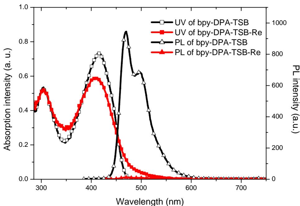
**Fig. S3.** Absorption and photoluminescence spectra in toluene solution for bpy-DPA-TSB (**6**) and bpy-DPA-TSB-Re (**7**) at 298 K.
