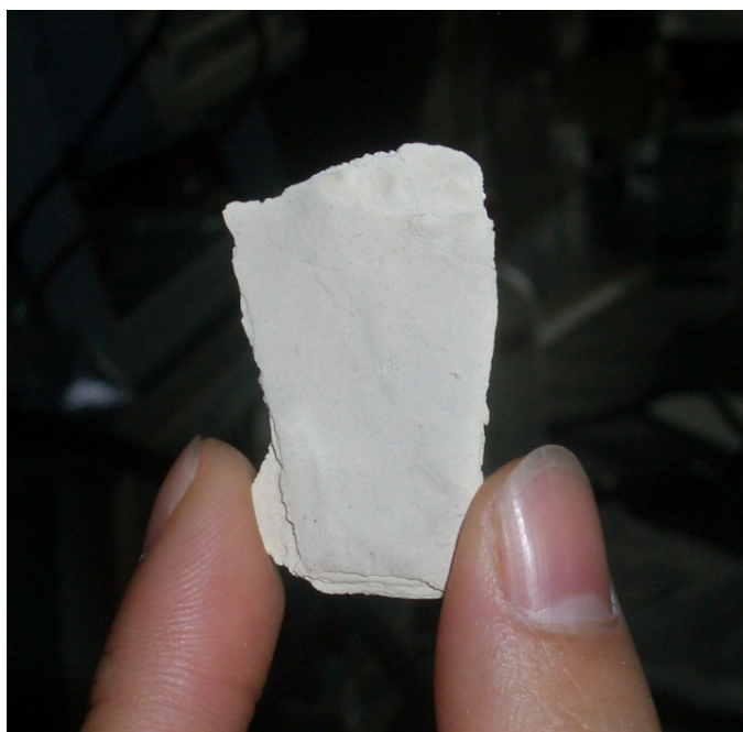
Figure S2. Photograph of self-supporting TiO 2 film prepared by combination of electrospinning method with hydrothermal approach.
