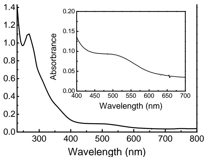
**Figure S3** UV/Vis spectrum of the complex, [Fe(*cis*-CO)<sub>2</sub>L] in methanol.
