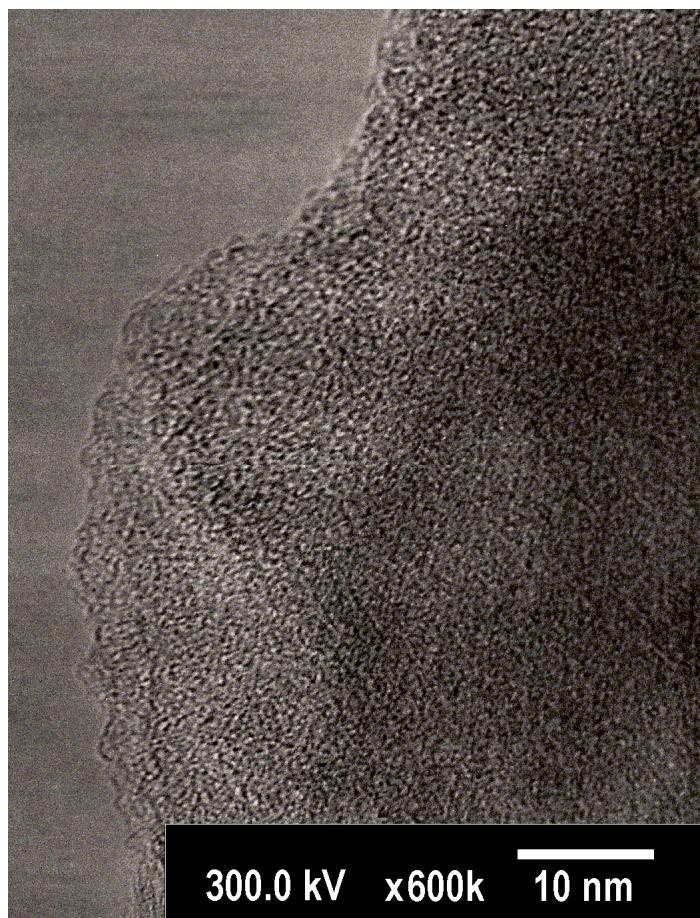
Figure 7. HRTEM image of OFP-3 illustrates its porosity (Wormhole structure), homogeneity, and structural stability under the experimental condition (300 kV). The pore dimensions in good agreement with the micropore size distribution as calculated by the Horvath-Kawazoe method.
