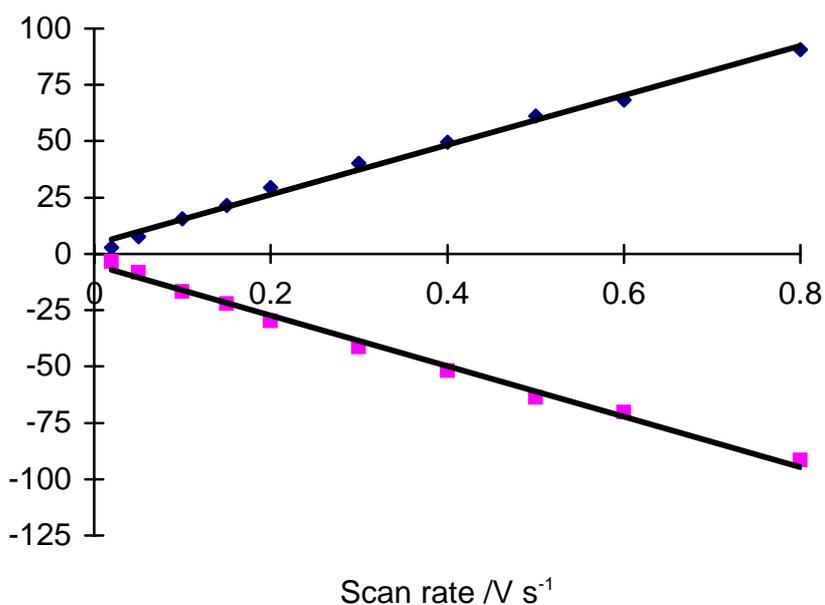
**Figure S3:** Peak current *versus* the scan rate for the cyclic voltammograms after the
