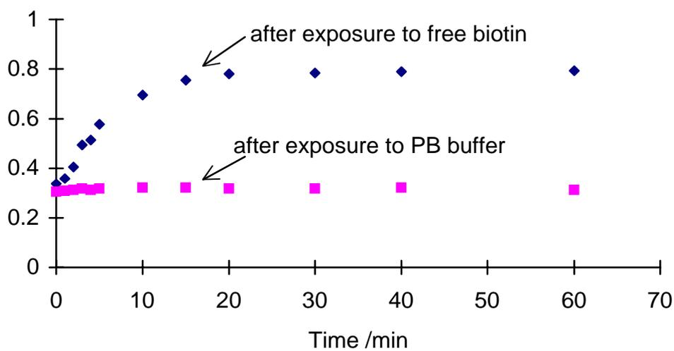
**Figure S10:** Relative current of anti-biotin modified GC surface after exposure of 0.3 mg mL<sup>-1</sup> biotin in 0.05 M phosphate buffer (pH 7.0) for different time and after
