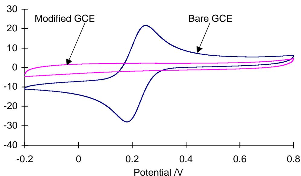
**Figure S2:** Cyclic voltammograms of the bare and mixed monolayer of MW and PEG modified GC electrodes in ferricyanide solution (1 mM; KCl, 0.05 M; phosphate buffer; pH 7.0) at a scan rate of  $100 \text{ mV s}^{-1}$  demonstrating the passivation of the electrode by the reductively adsorbed layer.
