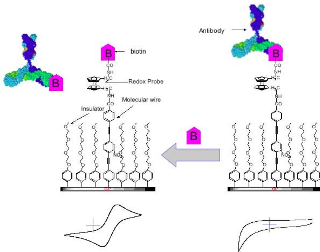
**Figure S9:** A schematic of the immuno-biosensor for detecting small molecules.
