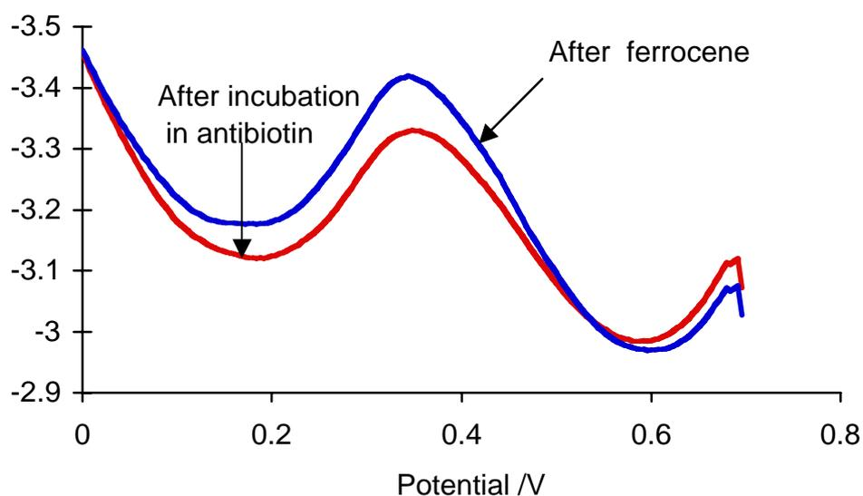
**Figure S6:** The response of the electrode before and after exposure to  $0.5 \mu\text{M}$  anti-biotin when there is no biotin attached to the end of the ferrocene. The only slight attenuation in current upon exposure of the anti-biotin demonstrates the ability of the interface to resist non-specific binding of the antibody.
