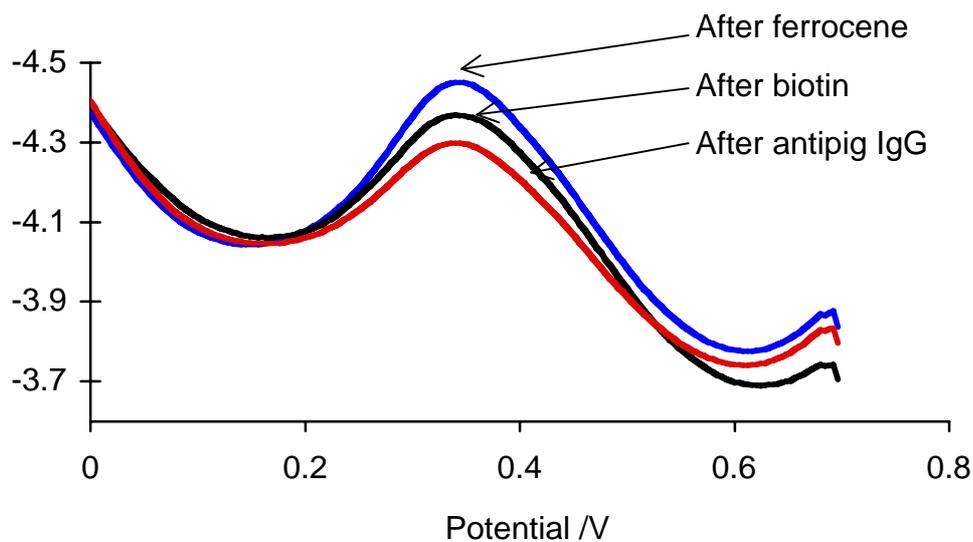
Figure S7: The response of the electrode a) after attachment of ferrocene dimethylamine, b) after attachment of biotin, and c) after exposure to 0.5  $\mu\text{M}$  anti-pig IgG antibodies that are not selective for biotin. The only slight attenuation in current upon exposure of the anti-pig IgG antibodies demonstrates the ability of the interface to resist non-specific binding of the antibody.
