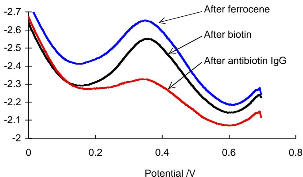
**Figure S4** Osteryoung Square Wave Voltammetry (OSWV) of the mixed monolayer of MW and PEG modified GC surfaces after the step-wise attachment of ferrocenedimethylamine, biotin and 0.5  $\mu\text{M}$  anti-biotin in 0.05 M phosphate buffer (0.05 M KCl, pH 7.0) at a scan rate of 100  $\text{mV s}^{-1}$ . This is comparable data to that shown in Figure 2a.
