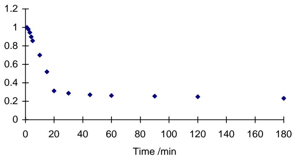
**Figure S8** Relative current from the OSWV for the biotin modified GC surfaces after incubation in 0.5  $\mu\text{M}$  anti-biotin for different incubation times. Relative current is obtained by dividing the current before the incubation of anti-biotin with the current after the incubation of anti-biotin.
