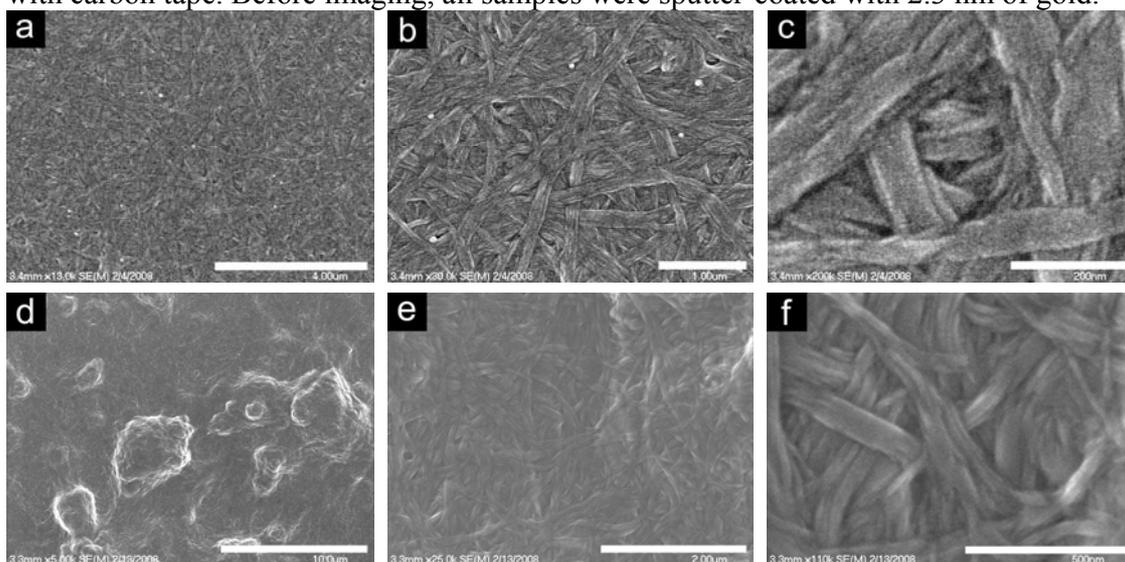
Figure S1. SEM images of the xerogel of **3** from decane gel (1.3 mM, images (a), (b), and (c), scale bars: (a) 4  $\mu\text{m}$ , (b) 1  $\mu\text{m}$ , and (c) 200 nm) and from TCE gel (10 mM, images (d), (e), and (f), scale bars: (d) 10  $\mu\text{m}$ , (e) 2  $\mu\text{m}$ , and (f) 500 nm).
