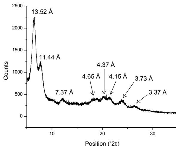
Figure S2. X-ray diffraction pattern for the xerogel of **3** from TCE.
