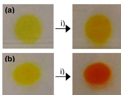
Figure S3. Cast film from rapid evaporation of TCE (a) and xerogel film (b) of **3** before and after i) exposure to the vapor of TFA for a few seconds. In the case of the cast film, extended exposure to the vapor of TFA did not change the color of the film.
