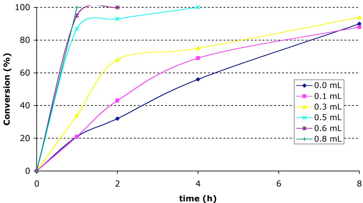
**Fig. 1.** Influence of the water volume for catalyst activation
